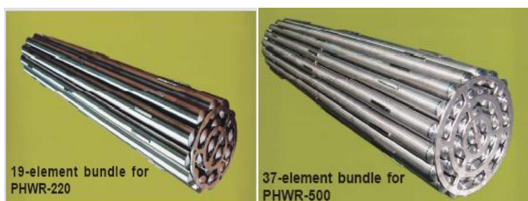
Figure 1: PHWR fuel bundles (a) 19-element for 220 MWe reactor, (b) 37-element for 540 and 700 MWe reactors
