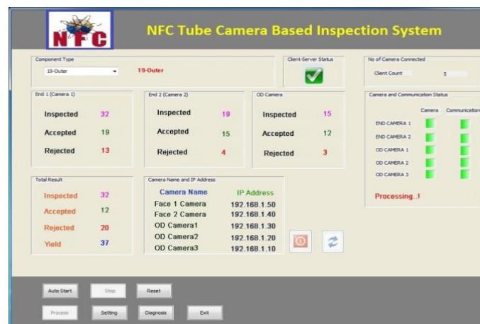
Figure 5: Operator screen in automatic tube inspection system
