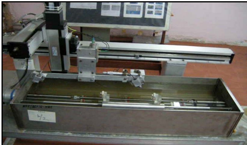
Fig. 3 Ultrasonic testing of PHWR end cap welds.
