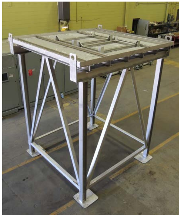
Figure 9 IFB-A Fuel Basket Transfer Platform (Pre-Delivery)
