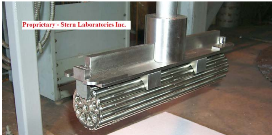
Figure 8 Fuel Bundle Handling Tool (Stern Laboratories Inc. supplied photo)
