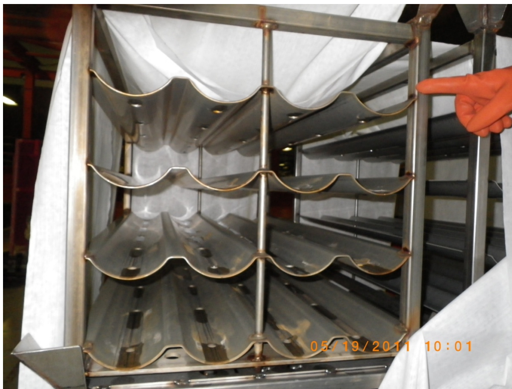
Figure 2 Standard Pickering Irradiated Fuel Bundle Storage Basket
