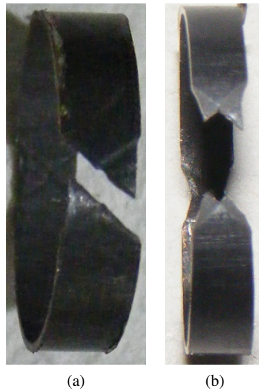
Figure 9: The photographs of the ring specimens of high burnup fuel clads tested at 583K showing (a) type I and (b) type II of failure.
