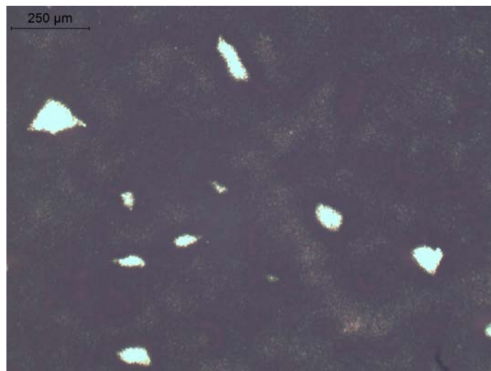
Figure 2 Alpha Autoradiograph of Archived Unirradiated BDL-422 (Th, Pu)O 2 Pellet. Light Areas are Pu-Rich Areas.
