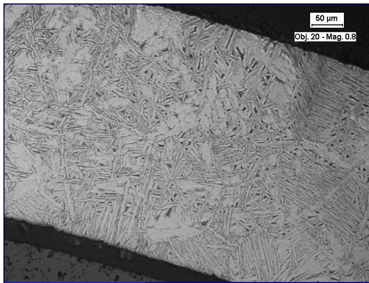
Figure 7 - Example of Heat-Affected Widmanstätten Microstructure
