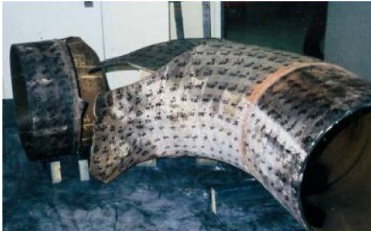
Figure 1 A Ruptured Elbow in Feedwater Line at Surry Unit 2(W. H. Ahmed [8])
