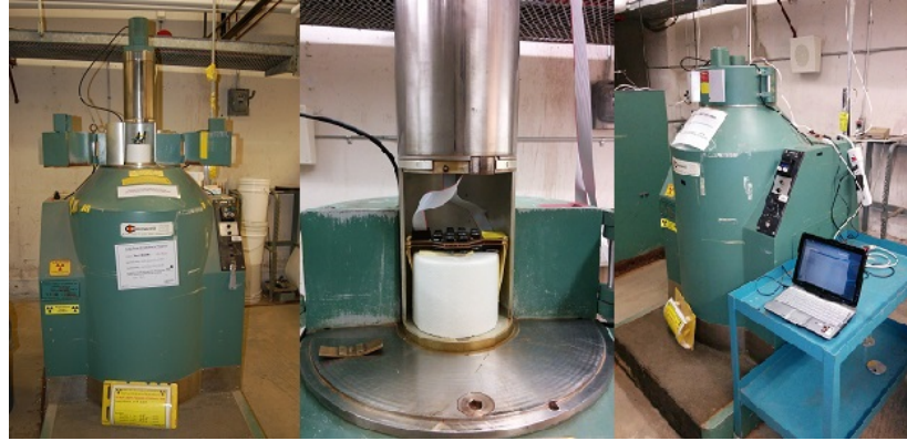
Figure 2 The Gamma-220 facility at CNL. Left: Chamber open for setup; Middle: Chamber zoom-in; Right: Chamber lowered and test started.
