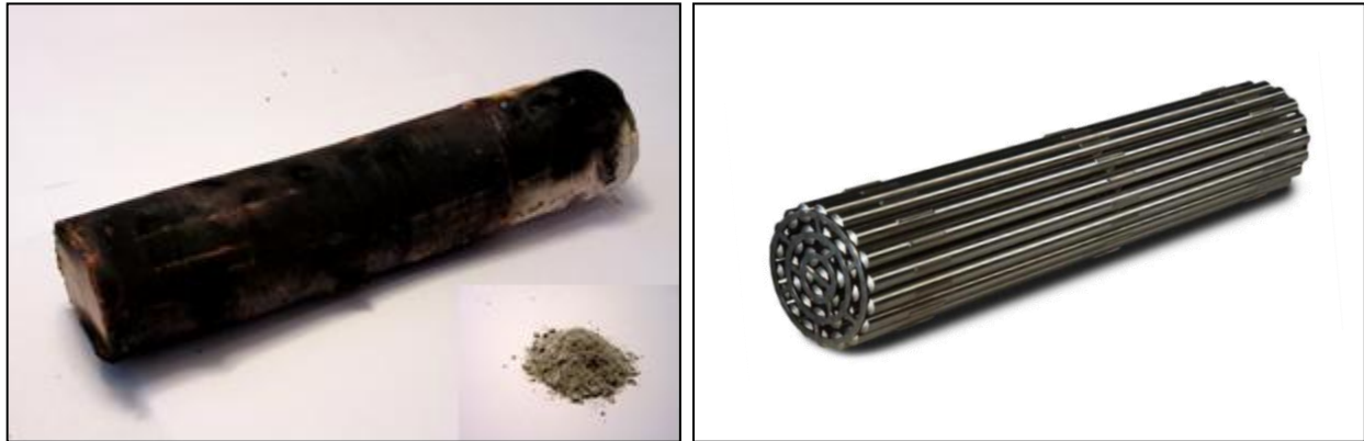
Figure 3. Incomplete Consumption of birch fuel log.
