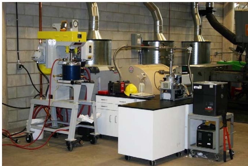
Fig. 1. Mechanical alloying facility (attrition mill and degassing unit) set up to process ODS steels.
