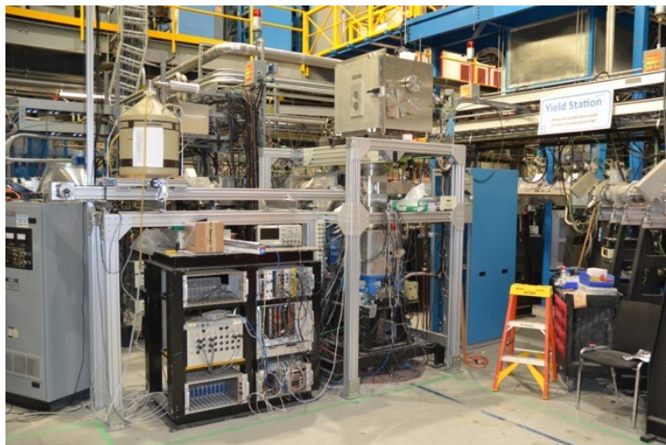
Figure 1 | High temperature tantalum target containers, as seen in Figure 1a, are filled with target material and then placed along the beam line, brought into the path of the protons to induce the collision reactions that generate the isotope beams studied at TRIUMF. The ISAC yield station seen in Figure 1b is used to characterize and diagnose isotope beams once they are generated and transported from the target module. The radioactive isotope beam comes in from below the experimental floor and is implanted onto an aluminized Mylar tape at the centre of the yield station. The isotope then decays and its identity is validated based on its decay curve and decay spectra [6].
