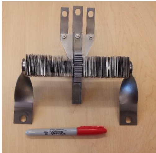
Figure 1 | High temperature tantalum target containers, as seen in Figure 1a, are filled with target material and then placed along the beam line, brought into the path of the protons to induce the collision reactions that generate the isotope beams studied at TRIUMF. The ISAC yield station seen in Figure 1b is used to characterize and diagnose isotope beams once they are generated and transported from the target module. The radioactive isotope beam comes in from below the experimental floor and is implanted onto an aluminized Mylar tape at the centre of the yield station. The isotope then decays and its identity is validated based on its decay curve and decay spectra [6].
