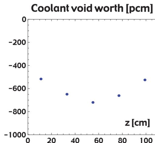
**Figure 2:** Axial distribution of void worth (pcm/22 cm slice).
