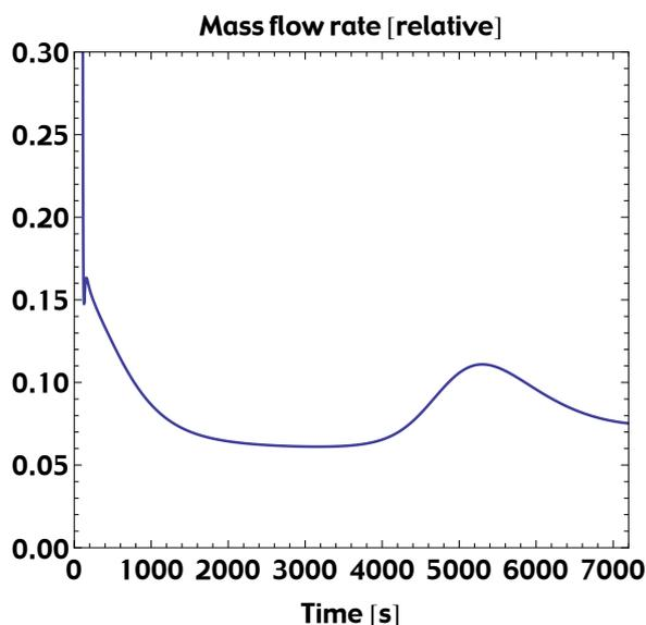
**Figure 7:** Coolant mass flow rate (relative to steady state operation) following an un-protected loss-of-flow accident at beginning of life.
