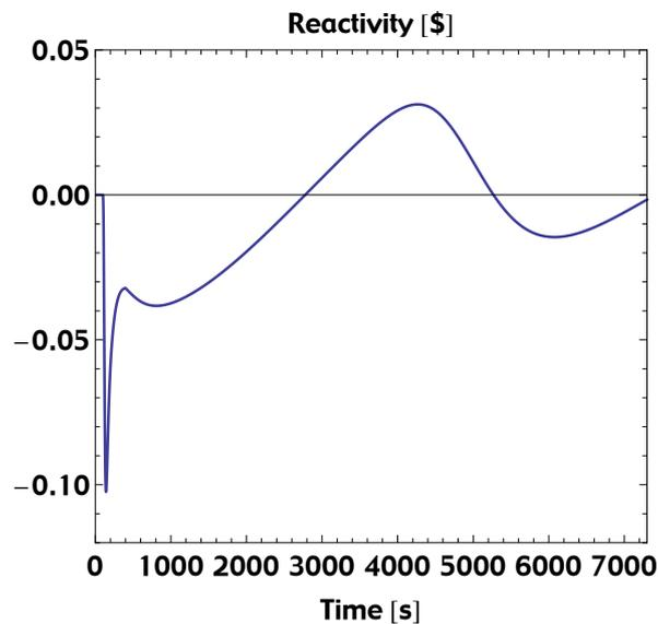
**Figure 6:** Reactivity evolution of the 3MWe SEALER core, following an un-protected loss-of-flow accident, at beginning of life.
