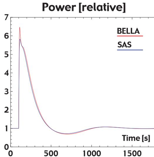
**Figure 3:** Predicted power evolution in the 3MWe SEALER core, following an un-protected reactivity insertion of 0.5\$ at beginning of life.
