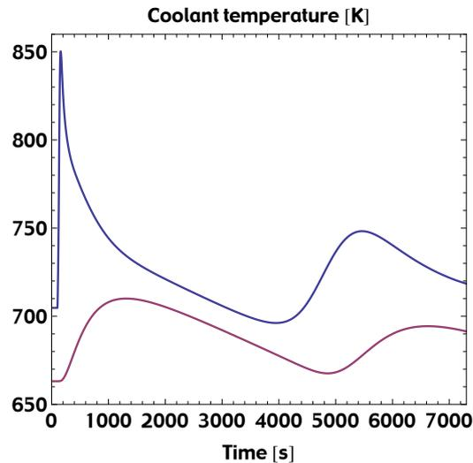
**Figure 5:** Coolant inlet (red line) and outlet (blue line) temperatures in the 3MWe SEALER system following an un-protected loss-of-flow accident, at beginning of life.
