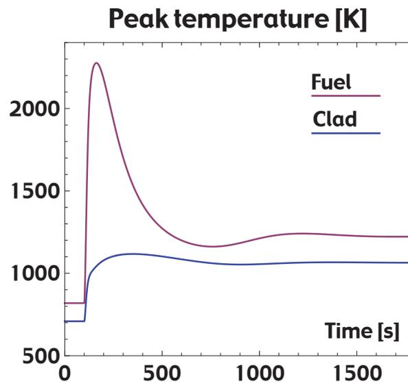
**Figure 4:** Peak fuel and clad temperatures in the 3MWe SEALER core following an un-protected reactivity insertion of 0.5\$ at beginning of life (SAS data).
