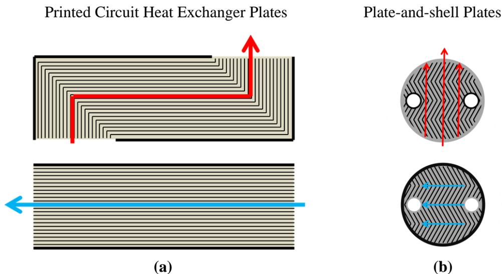
**Figure 2 (a) Examples of printed circuit heat exchanger plates (counter-cross-flow), and (b) examples of plate-and-shell plates (cross-flow). In printed circuit heat exchangers, each plate has a flat face and a grooved face, and adjacent plates are different. In Plate-and-shell heat exchangers, each plate is the same and the seals allow flow distribution from either the shell (top) or the ports (bottom).**
