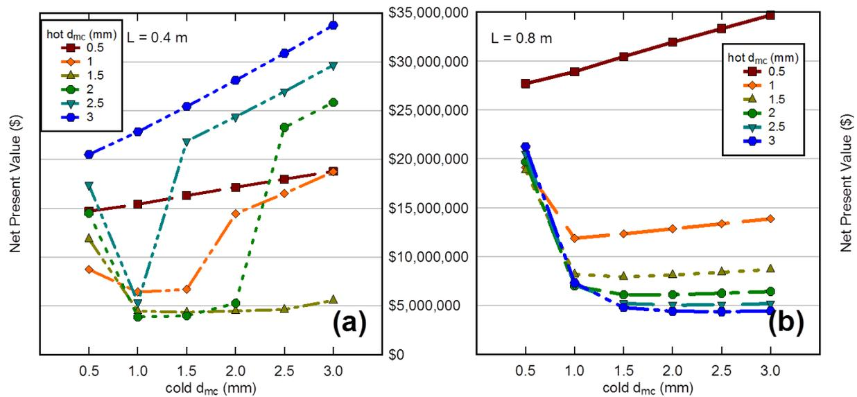
**Figure 6 Net Present Value vs minichannel diameter (cold fluid) for Printed Circuit Heat Exchangers. (a) Plate length of 0.4 m. (b) Plate length of 0.8 m.**
