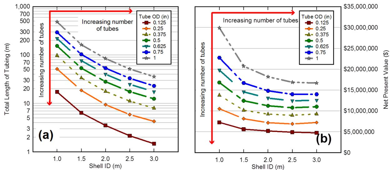
**Figure 4 (a) Total heat transfer length, and (b) Net Present Value vs Shell ID for Shell-and-Tube heat exchangers.**
