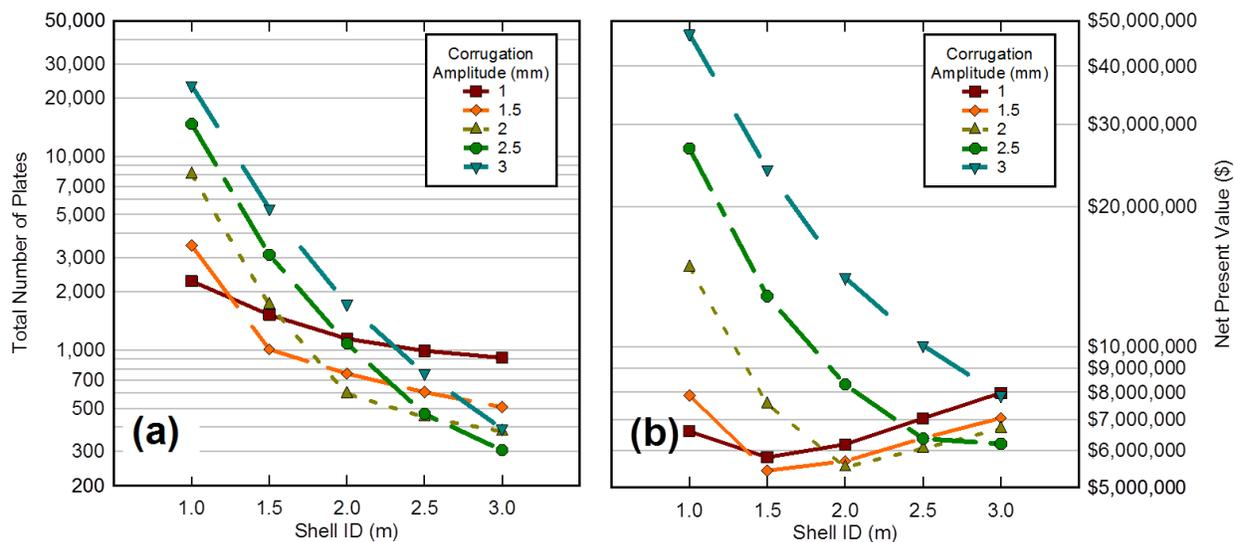
**Figure 5 (a) Total number of plates and (b) Net Present Value vs Shell ID for Plate-and-Shell heat exchangers.**
