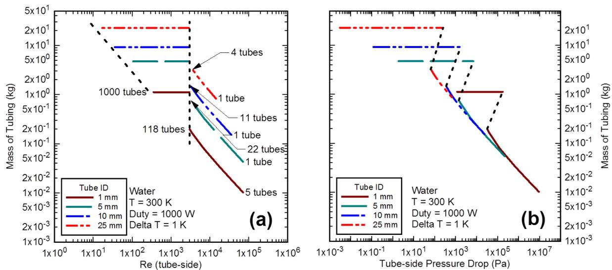
**Figure 1 (a) Calculated mass of tubing and (b) tube-side pressure drop for an example 1000 W heat exchanger.**
