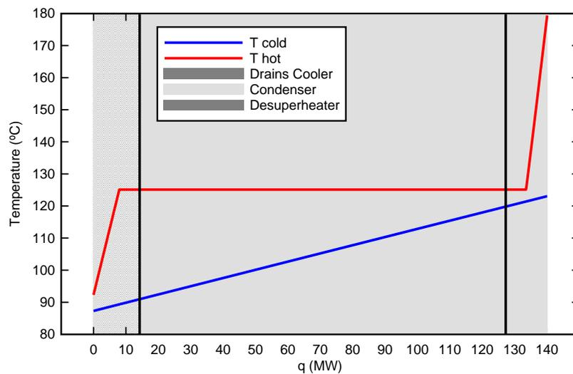
**Figure 3 T-q diagram of condensate heater used in the analysis.**
