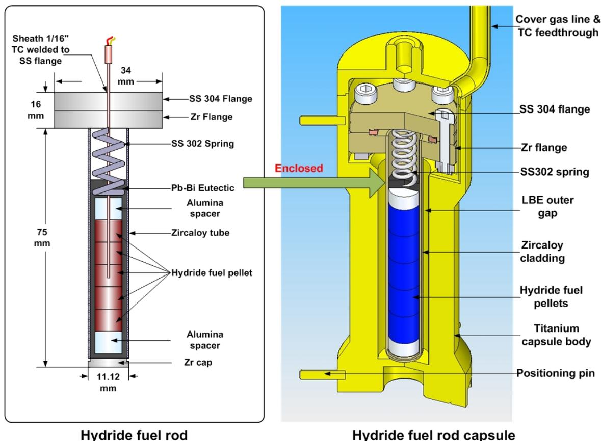
**Figure 6. The HYFI irradiation fuel sample (left) and irradiation capsule (right). The fuel samples were instrumented with a central thermocouple and an additional thermocouple on the clad outer surface (not shown).**
