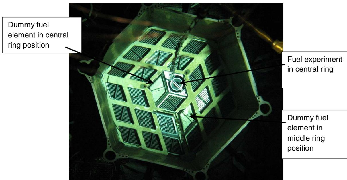
**Figure 1. A photograph showing the MITR core with a fuel experiment installed and the other two in-core experimental positions occupied by solid dummy elements as indicated.**
