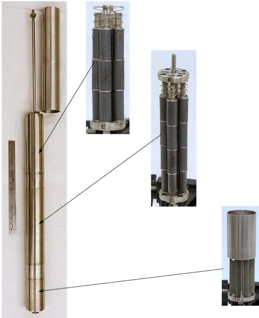
**Figure 3. In-core configuration for the Westinghouse Accident Tolerant Fuel irradiation. The sample stack shown on the left is composed of the three sample capsules as indicated.**
