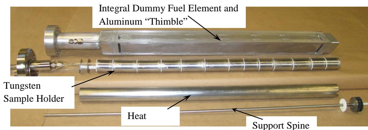
**Figure 7. Components of the very high temperature irradiation system. From the bottom of the dummy element to the flange is approximately 75 cm.**
