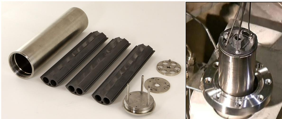
**Figure 5. The components of the flibe irradiation capsule (left) and the fully assembled capsule as it was being inserted into the irradiation facility (right). The sample cavities in the graphite segments contained material samples covered with flibe. Two thermocouples and inlet and outlet gas tubes were sealed into the capsule lid and can be seen in the right-hand photograph.**
