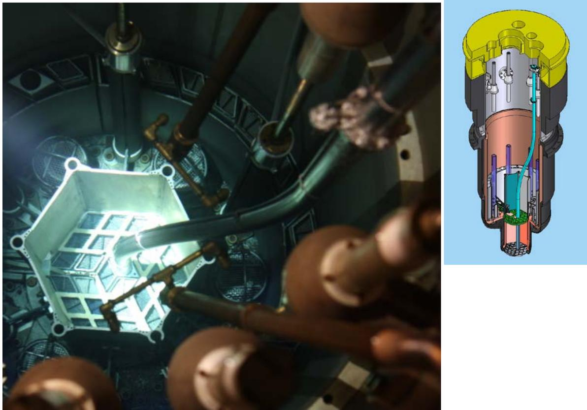
**Figure 4. A photograph (left) and 3-D rendering (right) of the In-Core Sample Assembly facility installed in the MITR.**
