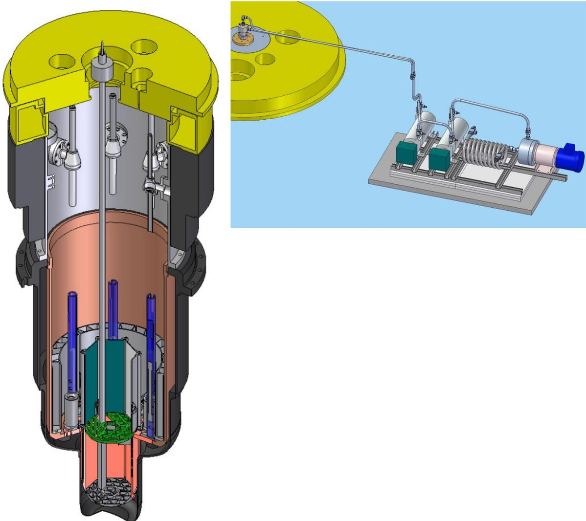
**Figure 2. Configuration of the in-core water loop in the reactor. On the left is the in-core containing thimble extending from the reactor top lid to the in-core position. On the right is the main circulating pump, dual heaters and regenerative heat exchanger positioned near the reactor core tank.**
