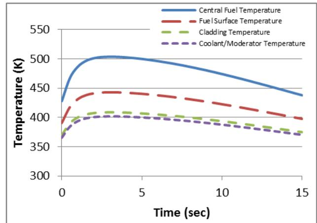
**Figure 10: Variation of the Average Reactor Component Temperature with Time for a +6.25mk Step Positive Reactivity Insertions**
