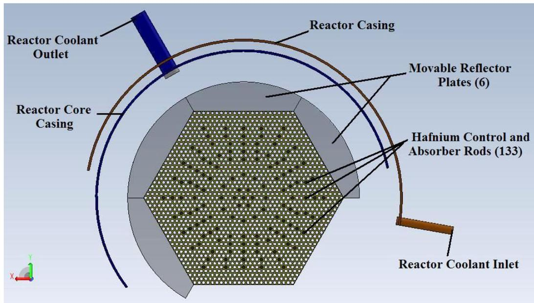
**Figure 2: SNB25 Nuclear Reactor Top View**
