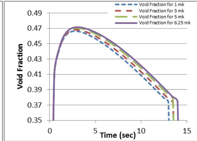
**Figure 8: Variation of the Void Fraction with Time for Positive Step Reactivity Insertions**
