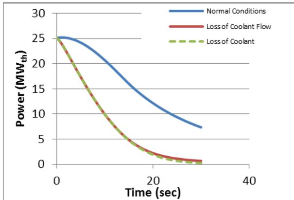
**Figure 11: Variation of Power with Time during Abnormal Conditions**
