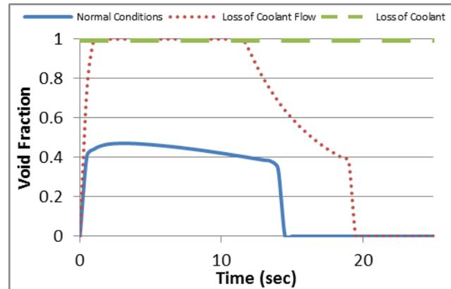
**Figure 12: Variation of Void Fraction with Time during Abnormal Conditions**
