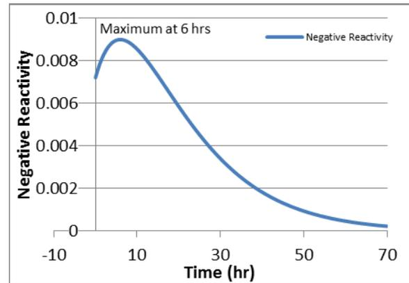
**Figure 16: Variation of Negative Reactivity with Time due to Xenon Buildup**
