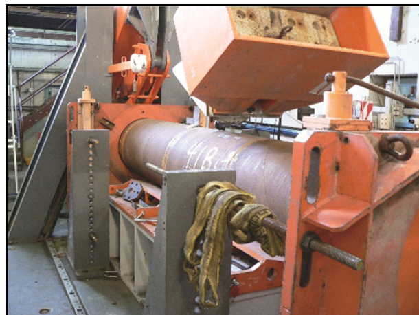
Figure 9 - GdF Suez lab simulates dents produced by a backhoe. Stress data obtained by neutron diffraction, will be useful to the industry in making hundred thousand-dollar decisions about how to manage pipelines that have sustained mechanical damage, for example, as a result of a backhoe digging in the wrong place.
