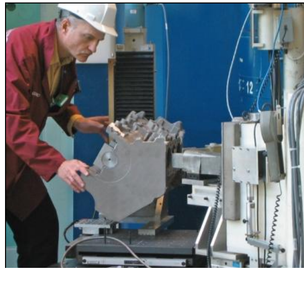
Figure 10 - NemaK prototype engine block installed on the L3 neutron stress scanner at the NRU reactor.
