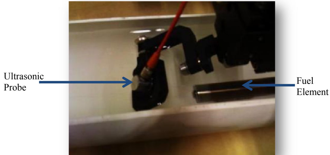
Figure 3: Inspection Set-up with Ultrasonic Probe Adjusted for Oblique Incidence
