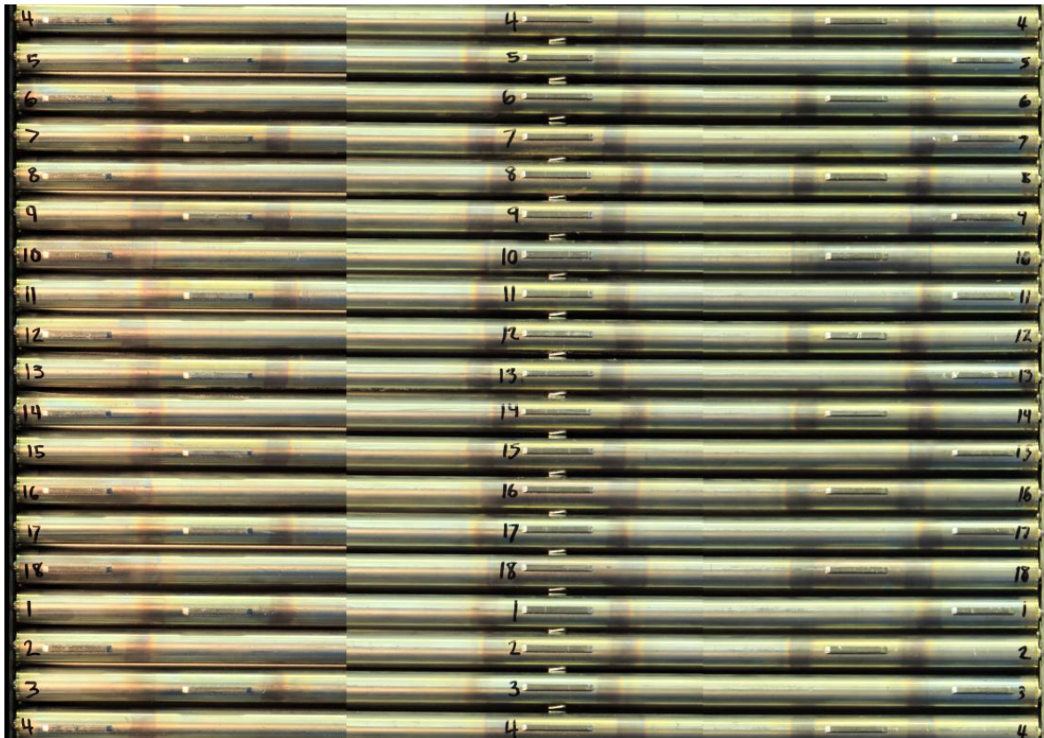
Figure 10 – An Example of the 'Unrolling' of the Video Taken During a Fuel Bundle Inspection. Provides full view of all outer elements.
