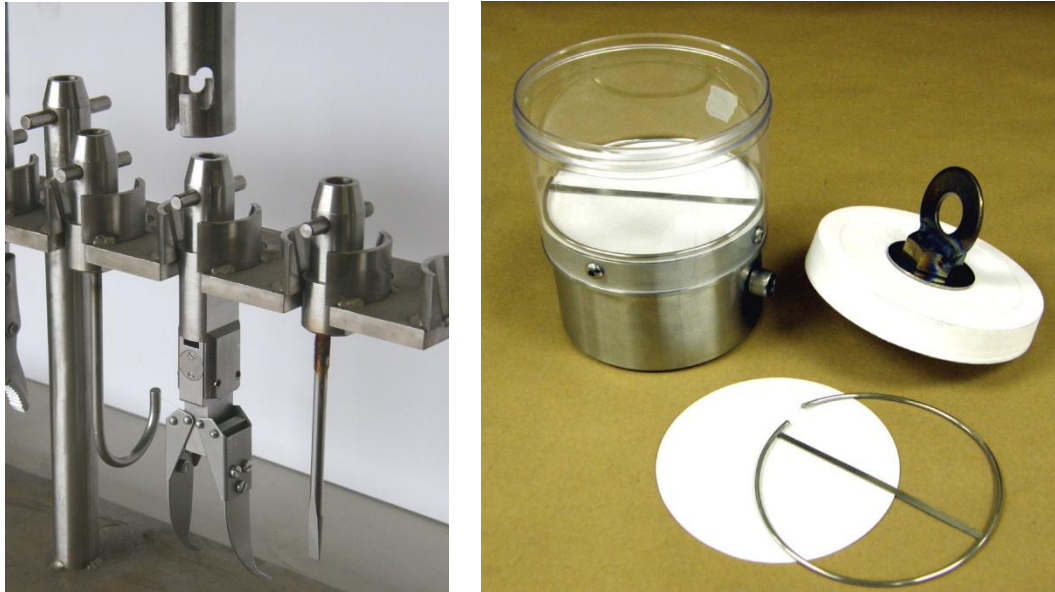
Figure 6 –Debris Collection Toolset Tweezers (left) and Debris Collection Bottle (Right)
