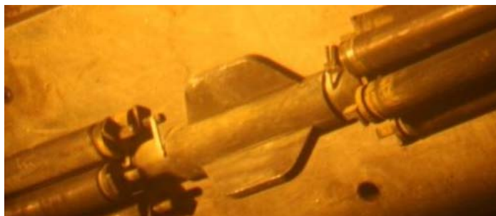
Figure 2 Periscopic view of the two tiers of fuel pins in the cluster
