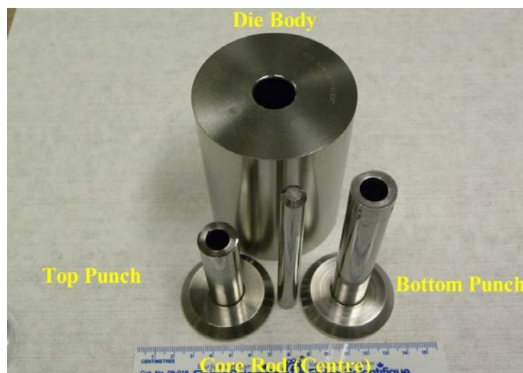
Figure 2: Annular Pellet Tooling
