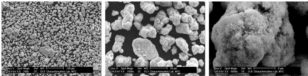
Figure 8 SEM microstructure of AU precipitated by 40 kg/hr ammonia flow rate
