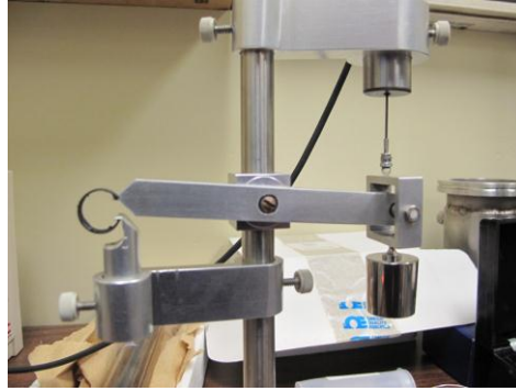
Figure 8: Apparatus for deflection testing
