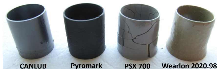
Figure 5: A second experiment was completed in a nitrogen atmosphere rather than in vacuum. Coatings cured in nitrogen and in vacuum appear structurally similar.
