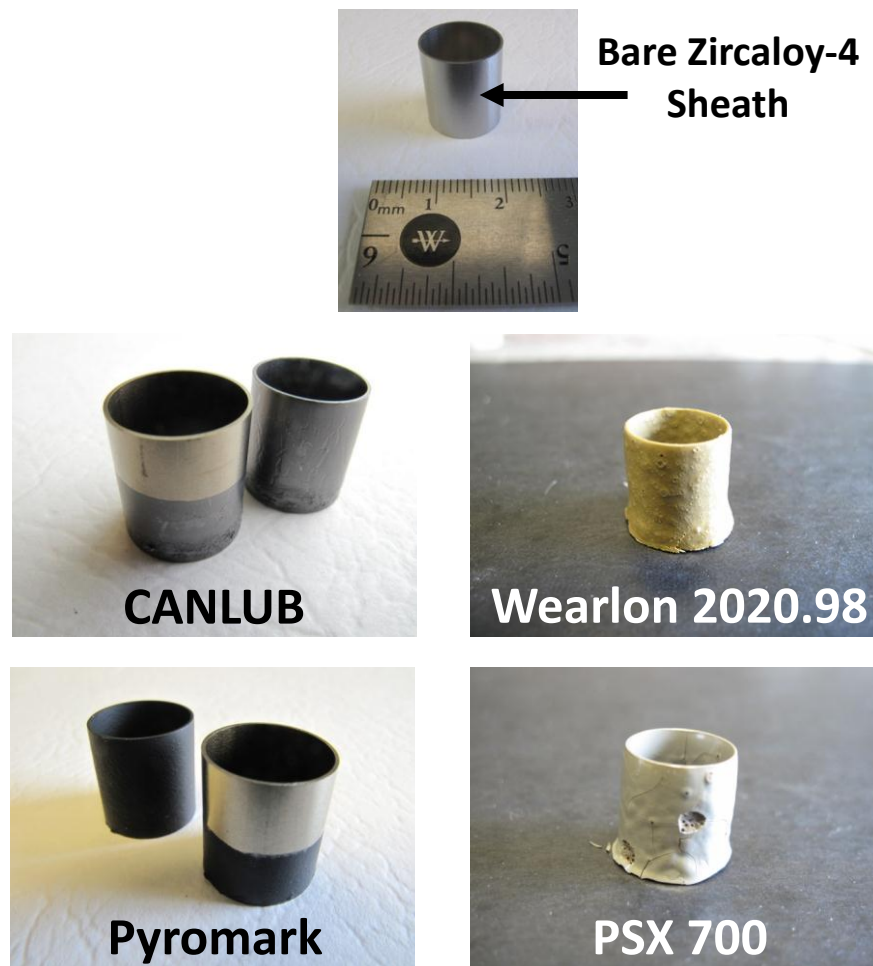
Figure 4: Uncoated Zircaloy-4 sheath sample, along with coated Zircaloy-4 sheath samples (after the coatings were baked). Half-coated samples facilitate the elemental analysis of uncoated and coated sections.
