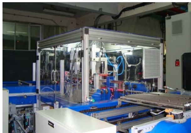
Fig.5: Automatic pellet visual inspection system
