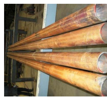
Fig. 11: As Extruded (119mm OD X 6mm Wt) Zr-2.5%Nb blanks
