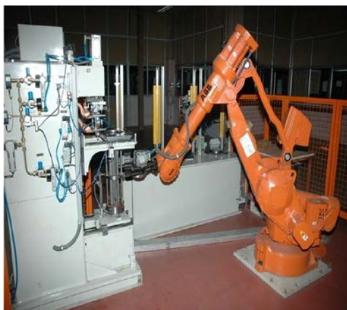
Fig.6: Industrial robot at endplate welding
