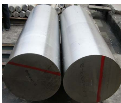
Fig. 9: 520 mm Ø Arc Melted and Machined Zr-2.5%Nb Ingots
