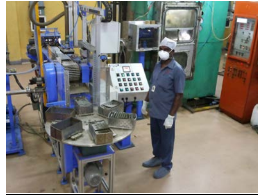
Fig.3: Mechanized pellet charging system
