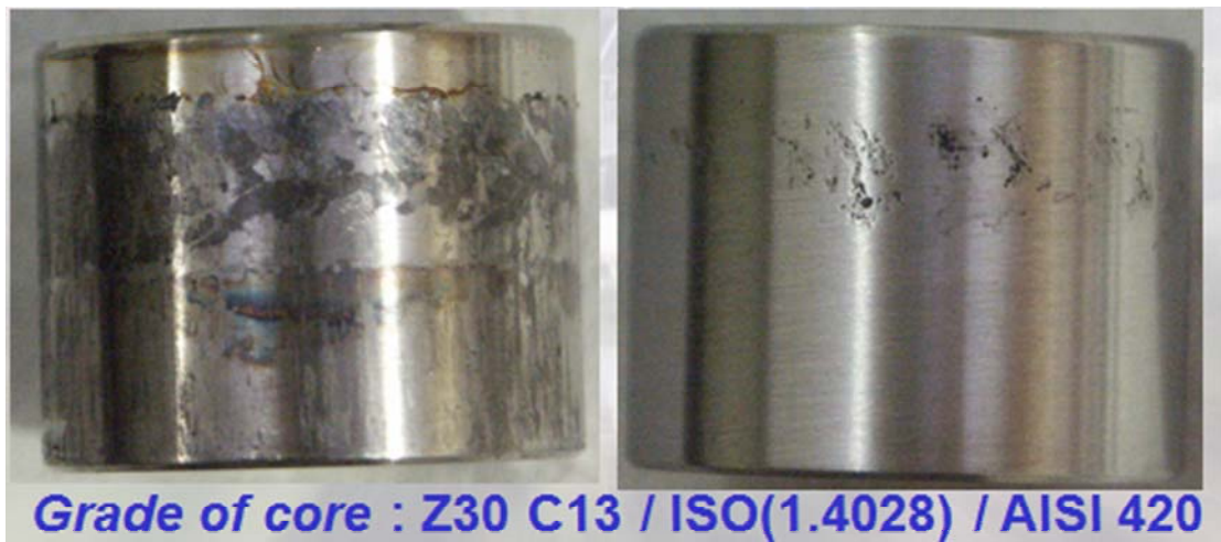
Figure 17. Z30 C13 Corrosion Comparison
