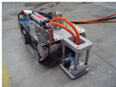
ACFM sensors carried out by a crawler
