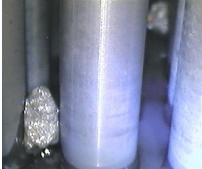
Figure 7: Foreign Objects Seen In-bundle from the Annulus Region
