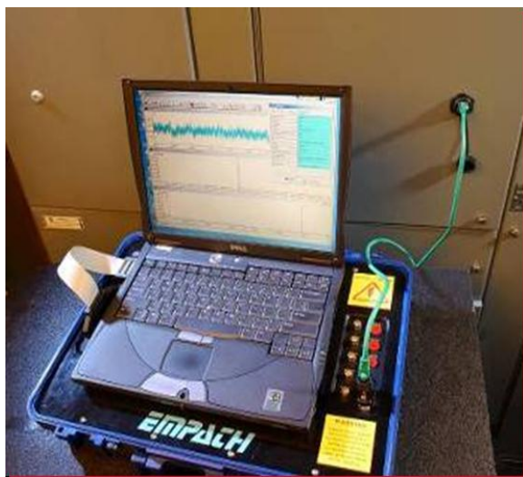
Figure 4: MCSA Tool EMPATH and Analysing Unit
