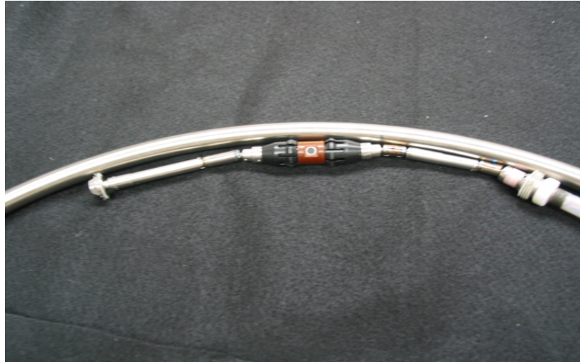
Figure 9. Rotating ultrasonic probe.
