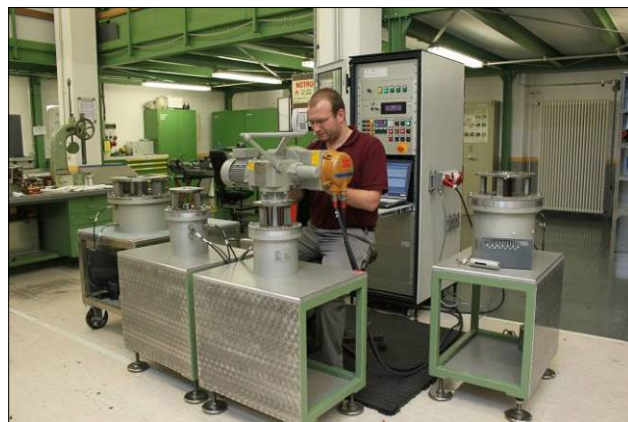
Figure 3 ADAM® system with MDP test benches and control panel in a workshop
