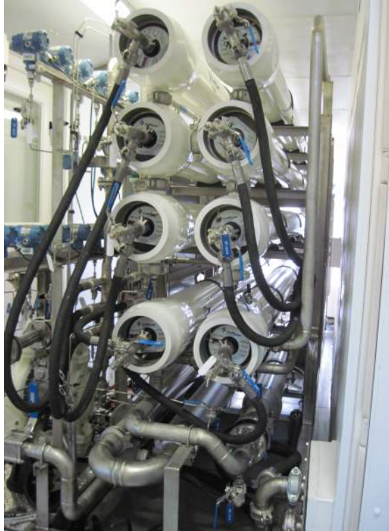
Figure 10: Westinghouse Mobile Reverse Osmosis Unit
