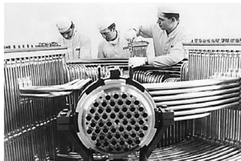
Fig. 8. Assembling the SG for the nuclear-powered cargo vessel Otto Hahn
