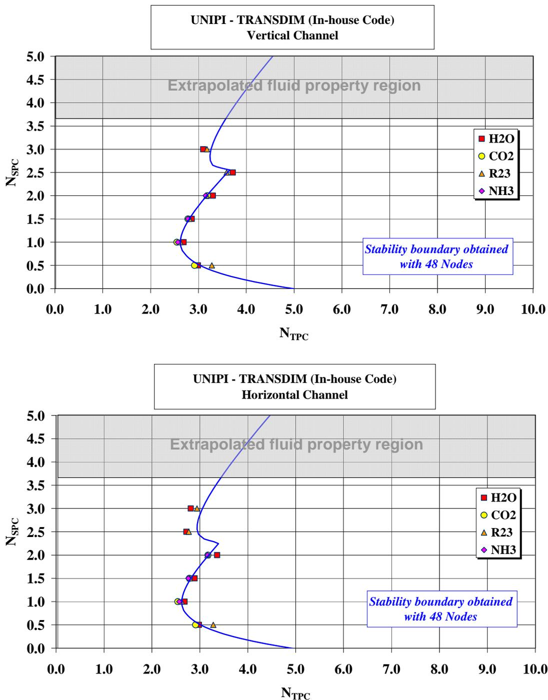
Figure 2. Reference data proposed for the second part of the benchmark exercise related to different fluids and vertical or horizontal channel [12]
