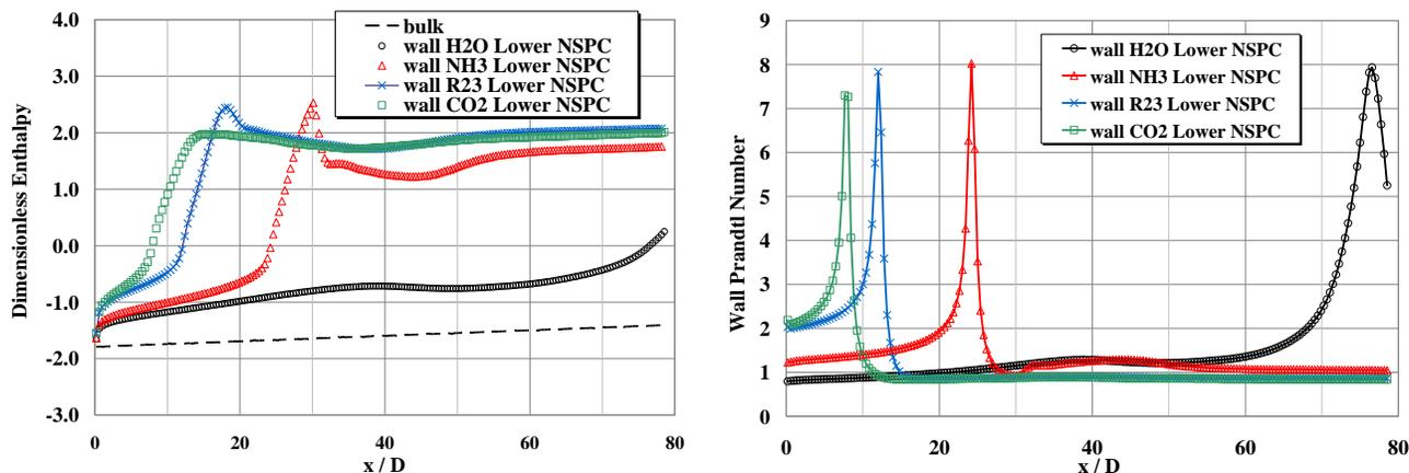
Figure 6. Bulk and wall dimensionless enthalpy and wall Prandtl number for the case with lower  $N_{SPC}$
