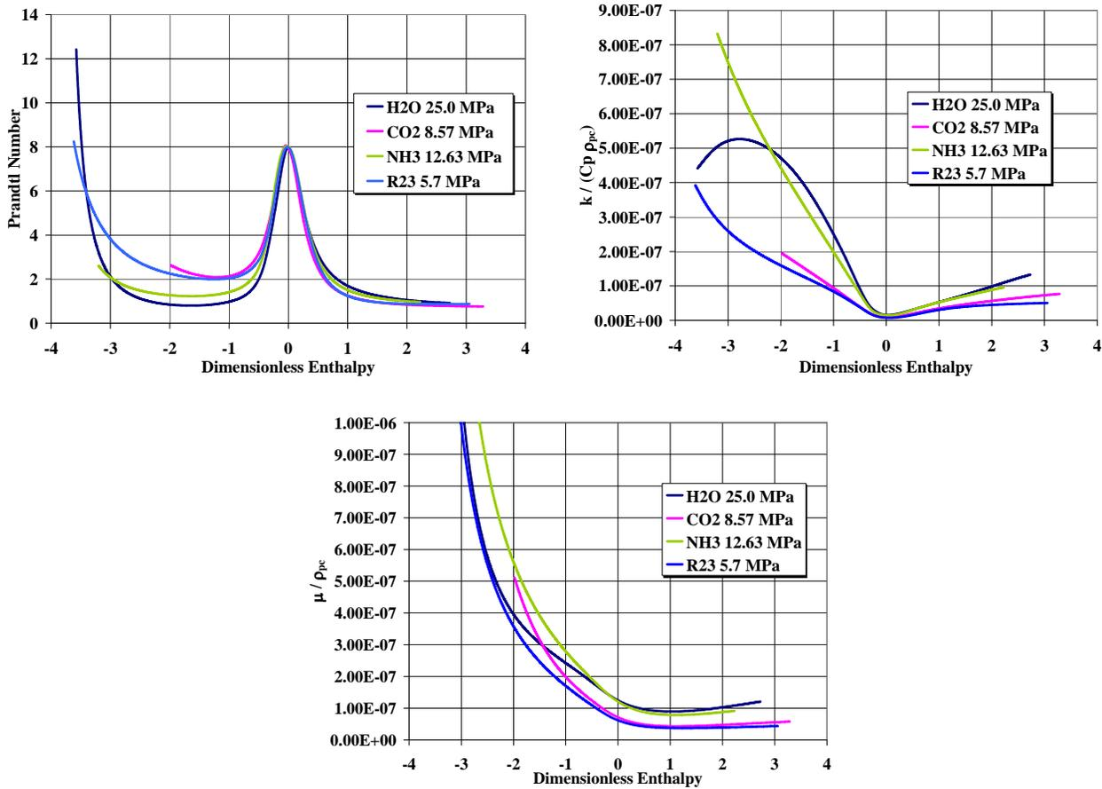
Figure 3. Prandtl number and reference diffusivities as a function dimensionless enthalpy for water, carbon dioxide, ammonia and R23 at different pressures
