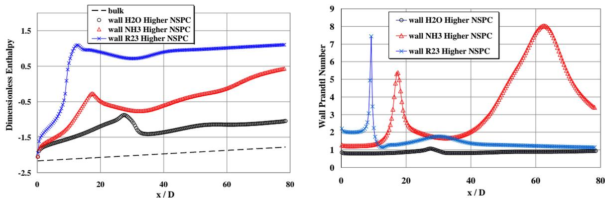
Figure 5. Bulk and wall dimensionless enthalpy and wall Prandtl number for the case with higher  $N_{SPC}$
