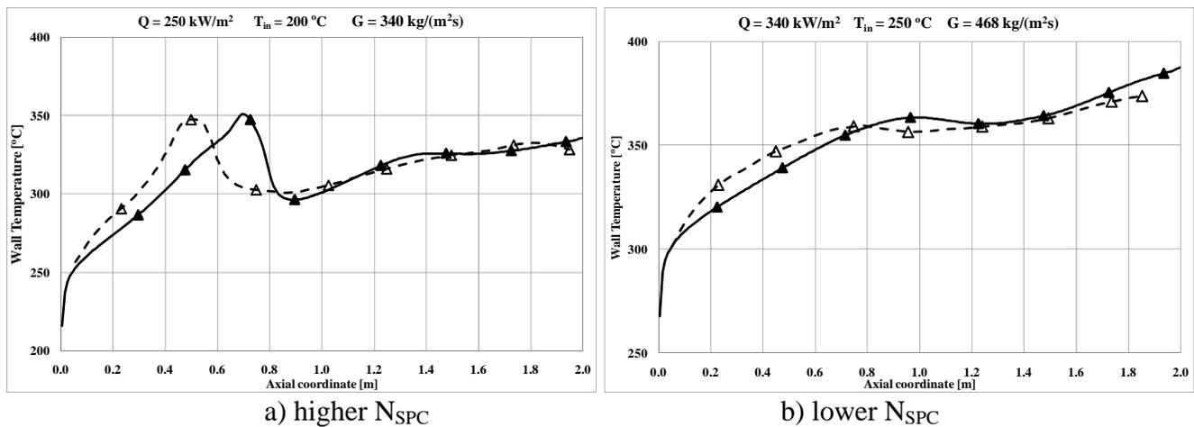
Figure 4. Calculated (continuous line) and predicted wall temperatures (dashed line) for the cases selected to be predicted with different fluids
