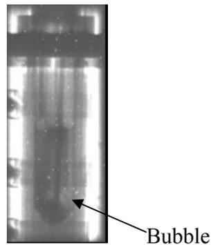
Fig. 3a. Large bubble at 45 °C with heavy water using ANDOR CCD camera (exp. time: 100 msec) at the ANTARES
