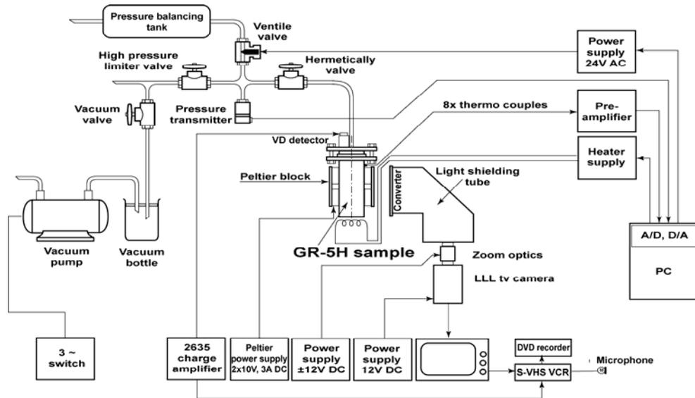
Fig. 2. Functional diagram of the measurement
