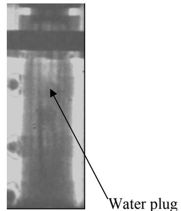
Fig. 4b. Water plug at 65 °C with heavy water using vidicon camera (exp. time: 40 msec) at the ANTARES.
