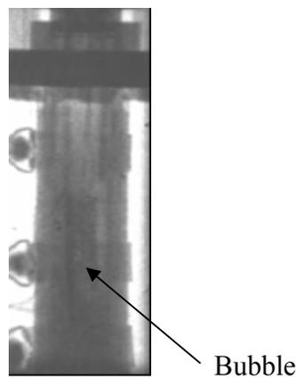
Fig. 4a. Large bubble at 50 °C with heavy water using vidicon camera (exp. time: 40 msec) at the ANTARES.
