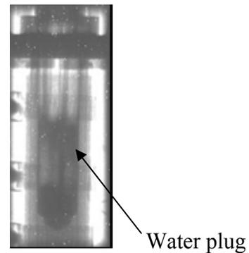
Fig. 3b. Water plug at 60 °C with heavy water using ANDOR CCD camera (exp. time: 100 msec) at the ANTARES
