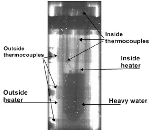
Fig. 1. Cold neutron radiography picture of GR-5H with 13 cm<sup>3</sup> heavy water at room temperature by ANDOR CCD camera
