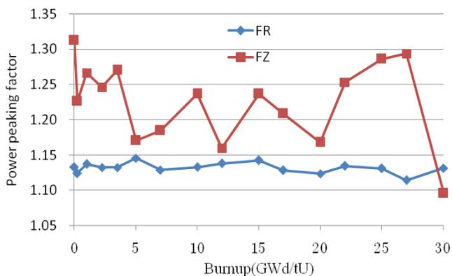
Fig. 8 Burnup profile of the power peaking factors
