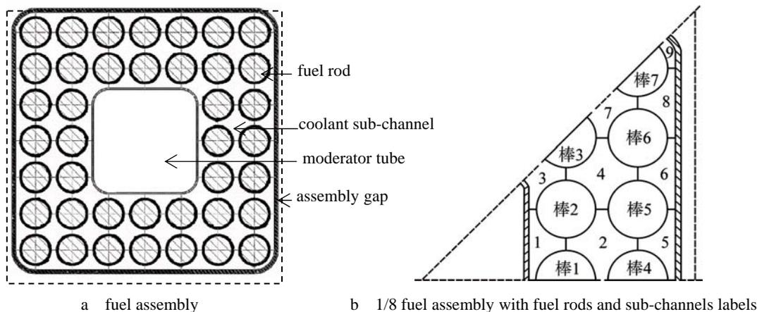
Fig. 2 Schematic Diagram of Full and 1/8 Assembly of HPLWR
