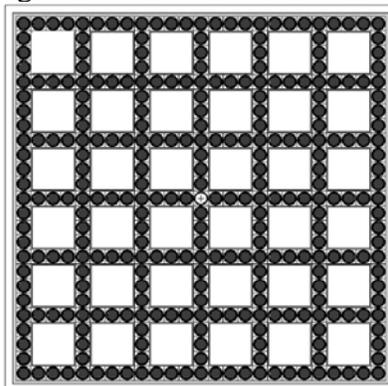
Fig. 6 Cross section of SCWR-H fuel assembly
