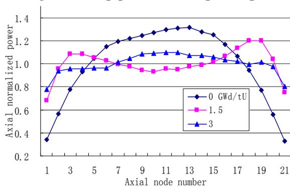
Fig.9 Horizontal averaged axial power distribution
