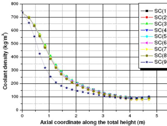
Fig. 4 Comparative Diagram of Axial Density Distribution in Sub-channels(MCATHAS vs. M-S)
