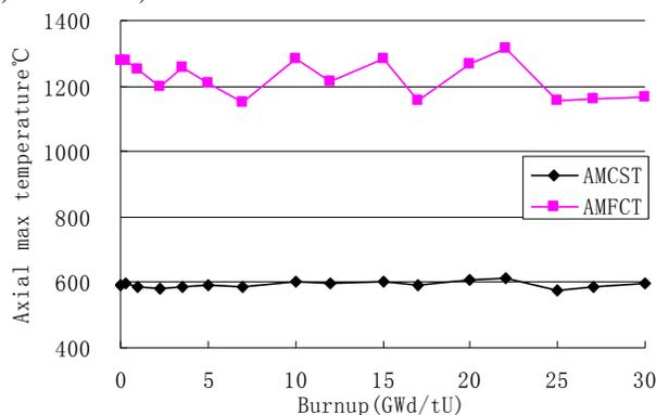
Fig. 10 Burnup profile of the AMCST and AMFCT
