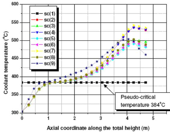
Fig. 3 Comparative Diagram of Axial Temperature Distribution in Sub-channels (MCATHAS vs. M-S)
