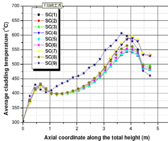
Fig. 5 Comparative Diagram of Axial Temperature Distribution of Cladding surface in the sub-channels (MCATHAS vs. M-S)
