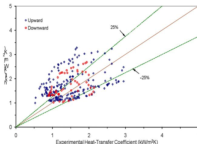
**Figure 13 Comparison of Experimental Heat Transfer Coefficient with the Predictions of the Krasnoshchekov Correlation for Upward and Downward Flow of Freon-22**
