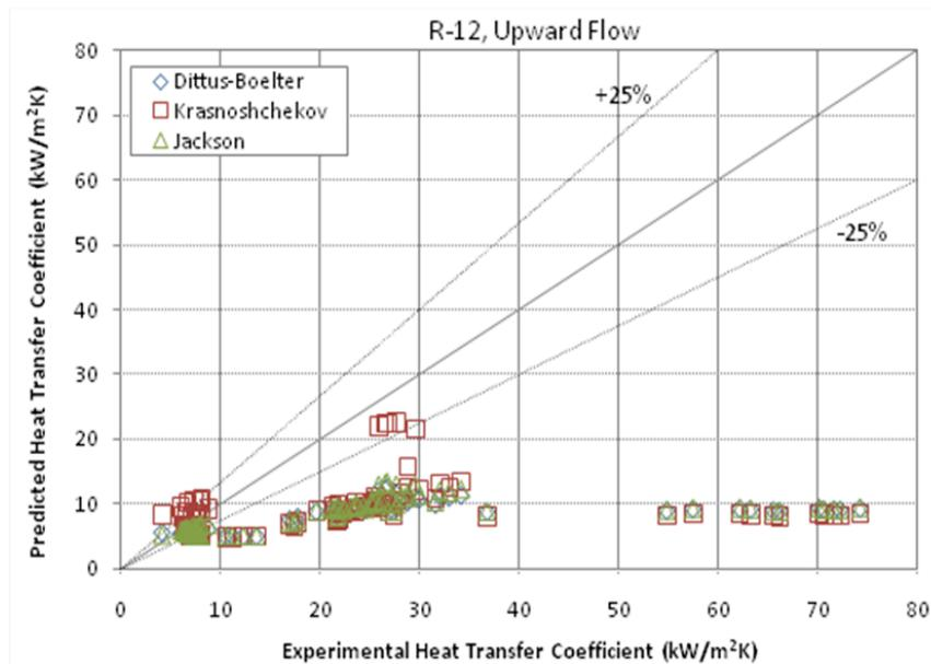
**Figure 9 Comparison of Experimental Heat Transfer Coefficient with the Predictions of the Correlations for Freon-12 Upward Flow**
