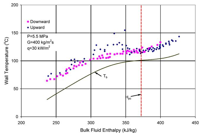
**Figure 6 The Effect of Flow Orientation in Bundles (Yamashita et al., 2006).**
