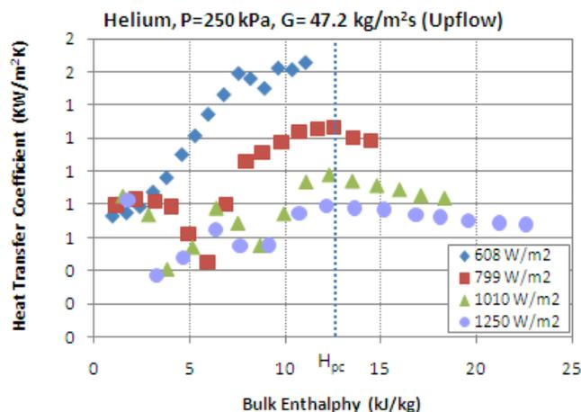
**Figure 2** Variation of Heat Transfer Coefficient With Bulk Enthalpy and Heat Flux (Bogachev, 1985).
