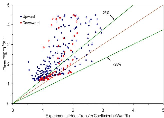
**Figure 12 Comparison of Experimental Heat Transfer Coefficient with the Predictions of the Dittus-Boelter Correlation for Upward and Downward Flow of Freon-22**
