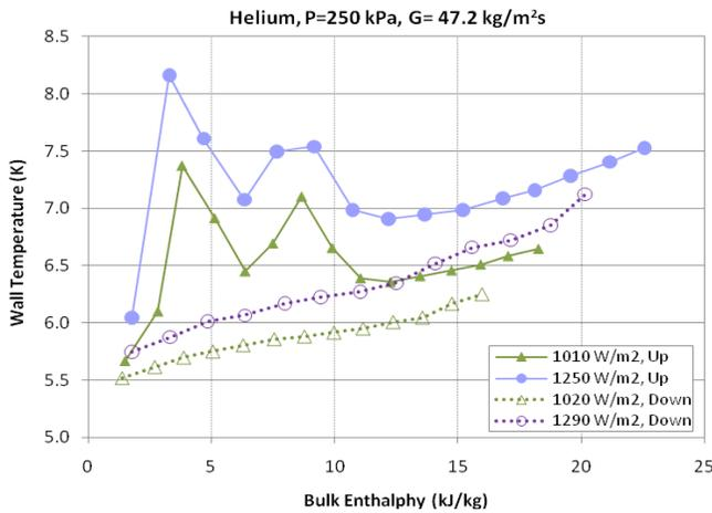
**Figure 3 Comparison of Upward and Downward Flow (Bogachev, 1985).**
