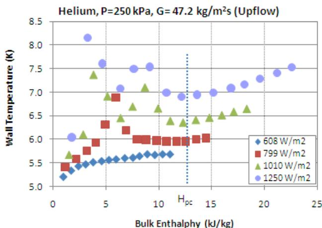
**Figure 1** Variation of the Wall Temperature With Bulk Enthalpy and Heat Flux (Bogachev, 1985).
