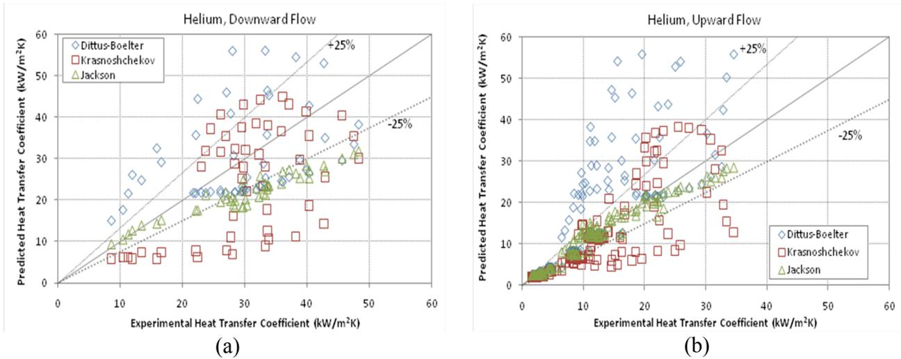
**Figure 10 Comparison of Experimental Heat Transfer Coefficient with the Predictions of the Correlations for Helium (a) Downward and (b) Upward Flows**
