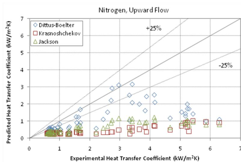
**Figure 11 Comparison of Experimental Heat Transfer Coefficient with the Predictions of the Correlations for the Nitrogen Upward Flow**
