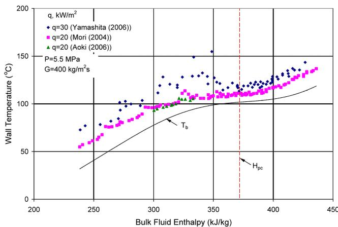
**Figure 5 Variation of the Wall Temperature with Bulk Enthalpy and Heat Flux in Bundles.**
