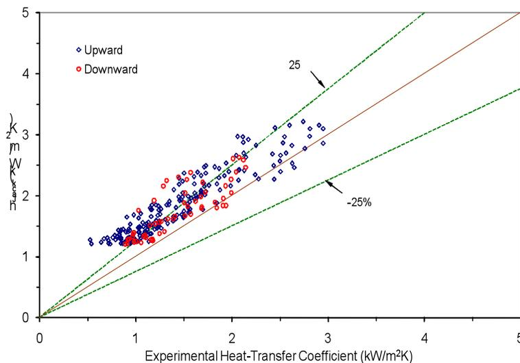
**Figure 14 Comparison of Experimental Heat Transfer Coefficient with the Predictions of the Jackson Correlation for Upward and Downward Flow of Freon-22**
