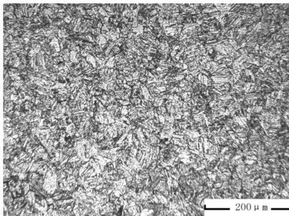
Fig. 7 Microstructure of CNS-II steel with 1000 °C/30 min/W.C. plus 780 °C/90 min/A.C. heat treatment
