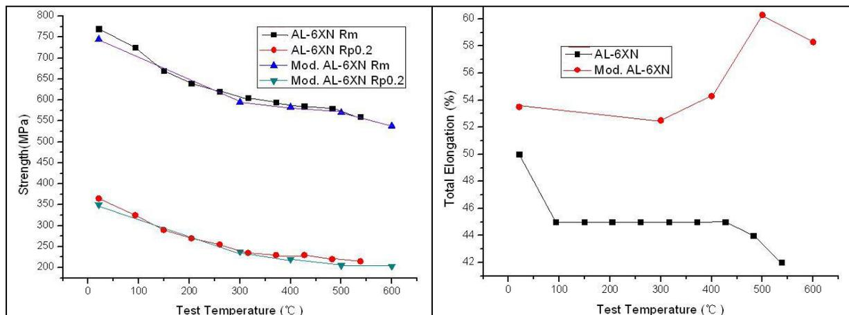
Fig. 2 Comparison of tensile properties between Mod AL-6XN and commercial AL-6XN steel
