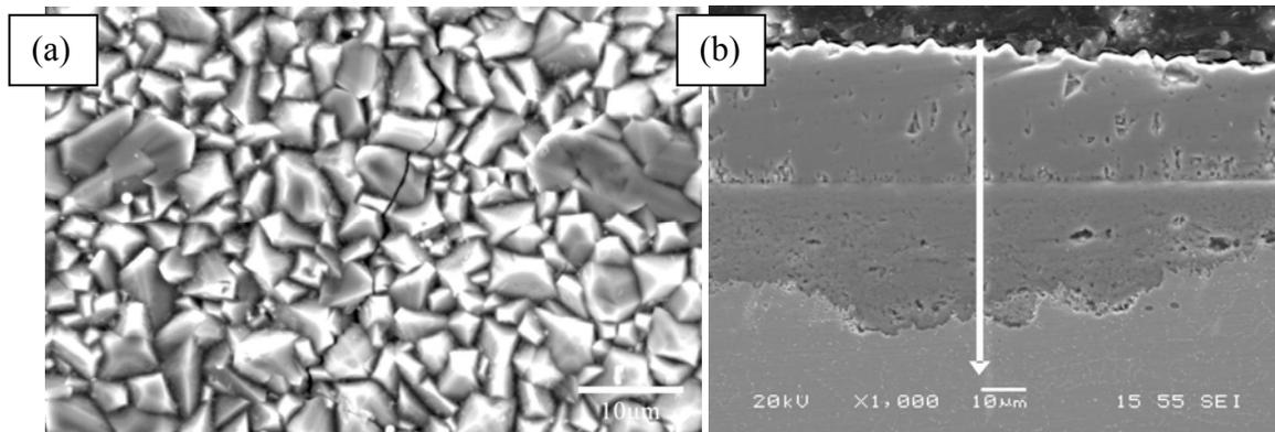
Fig. 9 SEM images of the surface morphology (a) and cross-section (b) of CNS-II exposed to SCW at 650 °C and 25 MPa for 1000 h
