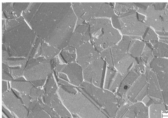
Fig. 1 Microstructure of Mod AL-6XN after solution treatment at 1100 °C
