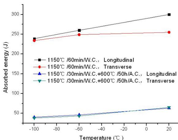
Fig. 3 Absorbed energy as a function of temperature under various conditions
