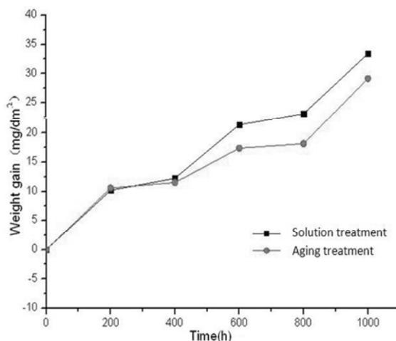
Fig.4 The weight gain of Mod AL-6XN exposed to SCW at 650 °C and 25 MPa
