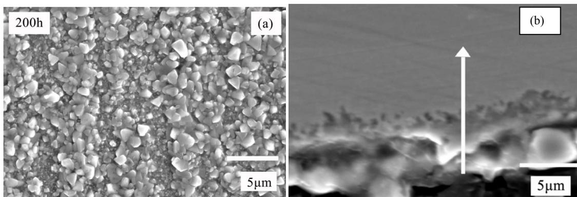
Fig.5. SEM images of the surface morphology (a) and cross-section (b) of Mod AL-6XN exposed to SCW at 650 °C and 25 MPa for 200 h and 1000 h, respectively.
