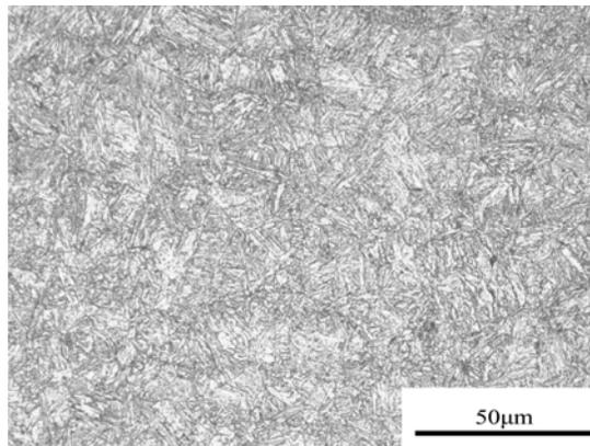
Fig. 6 Microstructure of CNS-I steel with 950 °C/30 min/W.C. plus 780°C/90 min/A.C. heat treatment
