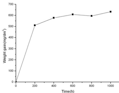
Fig. 8 The weight gain of CNS-II exposed to SCW at 650 °C and 25 MPa
