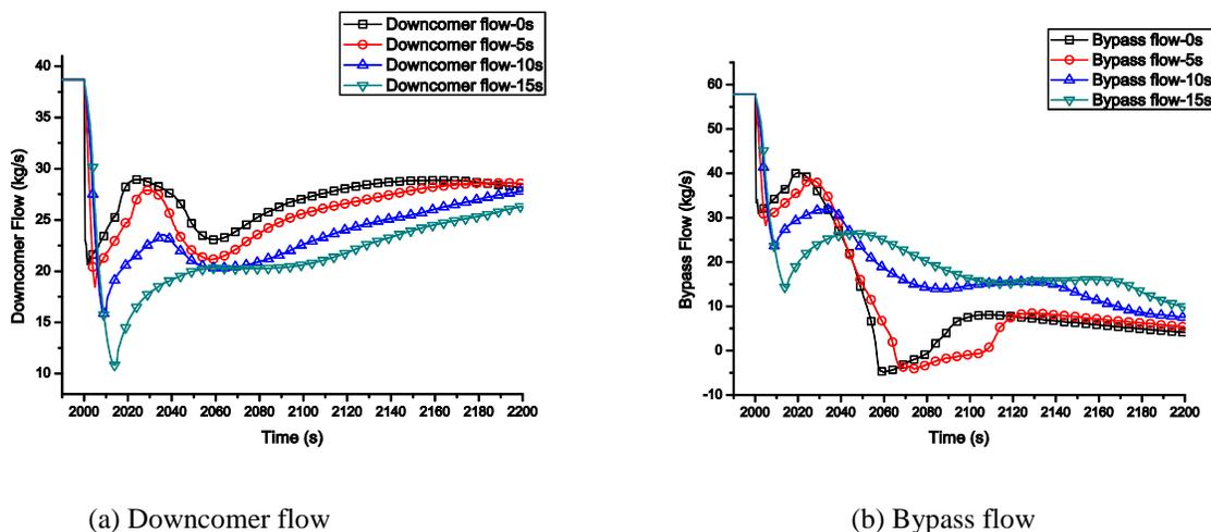
Fig. 6 Downcomer and bypass flow change with different coast-down time
