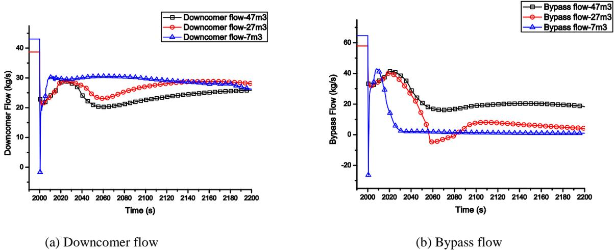
Fig. 9 Downcomer and bypass flow change with different RPV upper water volume
