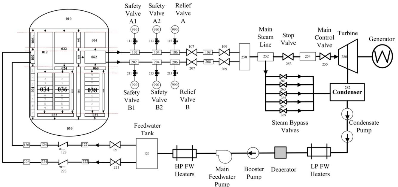
Fig. 1 SCWR-M system model node
