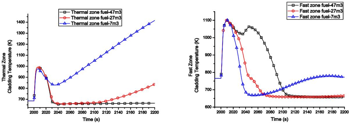
(a) Thermal zone cladding temperature
