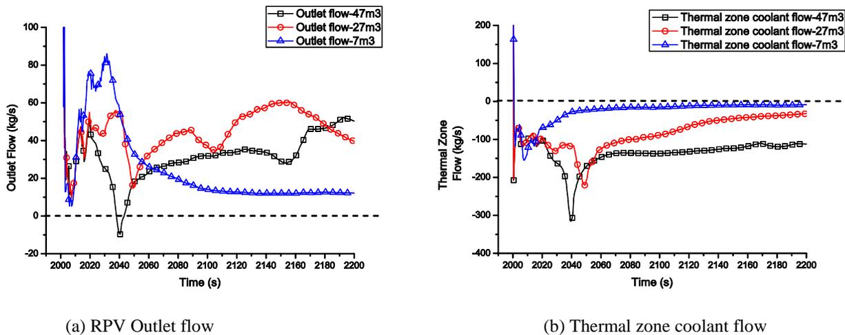
Fig. 10 Outlet and thermal zone coolant flow change with different RPV upper water volume
