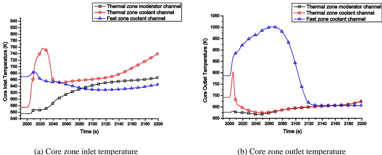
Fig. 3 Core in-out temperature during LOFT
