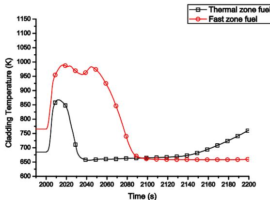
Fig. 5 Fuel cladding temperature during LOFT
