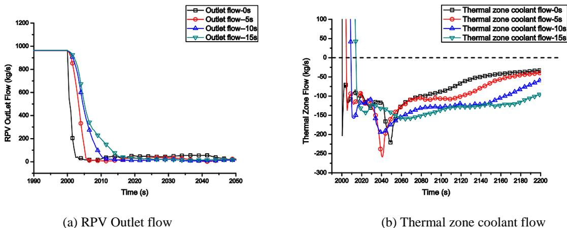
Fig. 7 Outlet and thermal zone coolant flow change with different coast-down time
