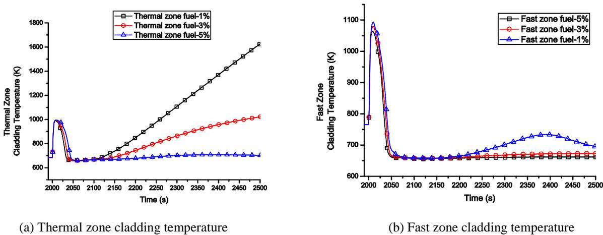
Fig. 14 Thermal and fast zone cladding temperature change with different safety injection flow
