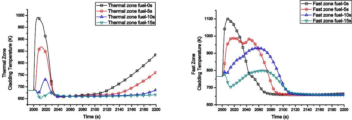
(a) Thermal zone cladding temperature
