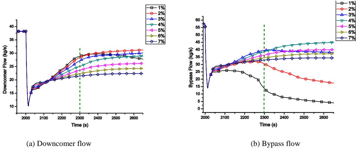
Fig. 12 Downcomer and bypass flow change with different safety injection flow
