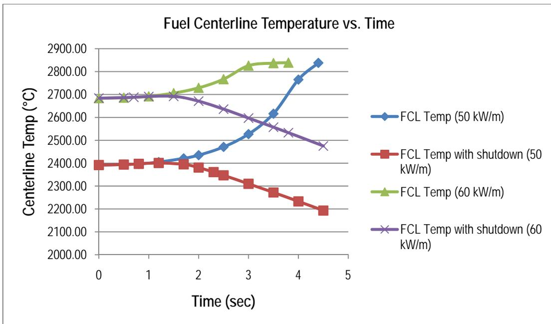
Figure 12: Fuel centerline temperature vs. time for 1 mk/s insertion rate
