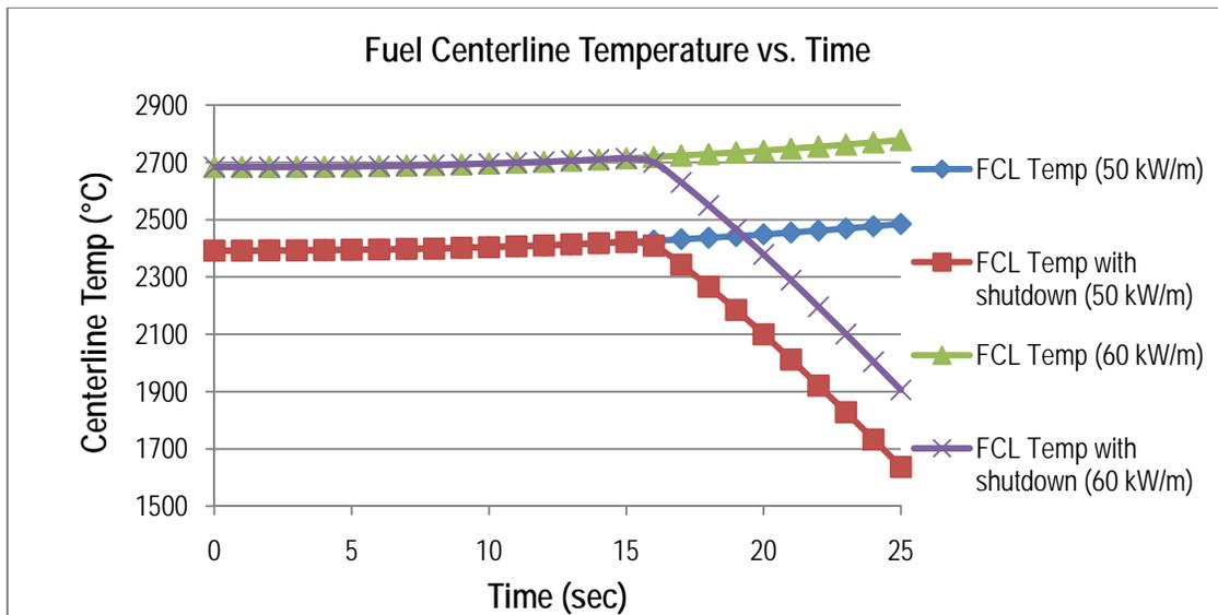
Figure 6: Fuel centerline temperature vs time for 0.01 mk/s insertion rate
