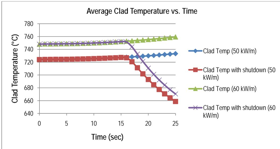
Figure 5: Average Clad Temperature vs time for 0.01 mk/s insertion rate
