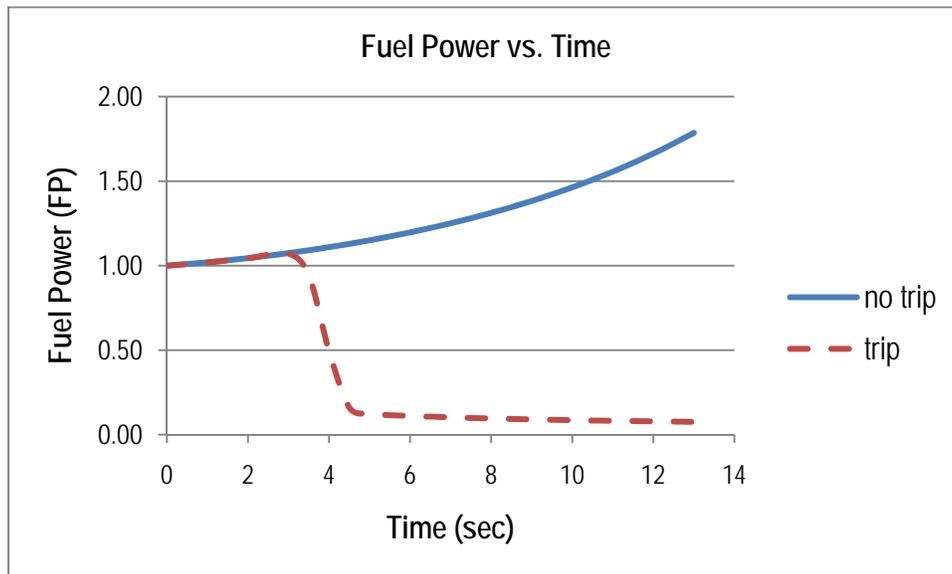
Figure 7: Fuel Power vs. Time for 0.1 mk/s reactivity insertion rate
