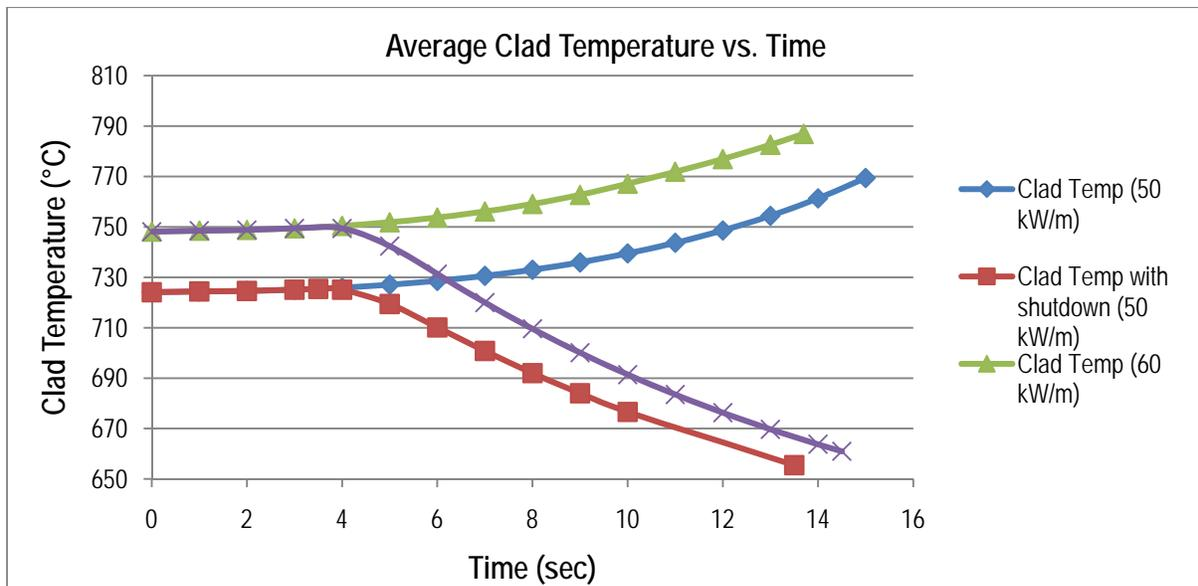
Figure 8: Average Clad Temperature vs. time for 0.1 mk/s insertion rate
