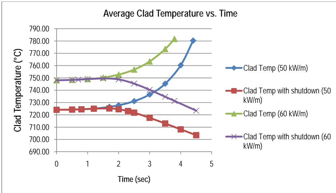
Figure 11: Average Clad Temperature vs. time for 1 mk/s insertion rate
