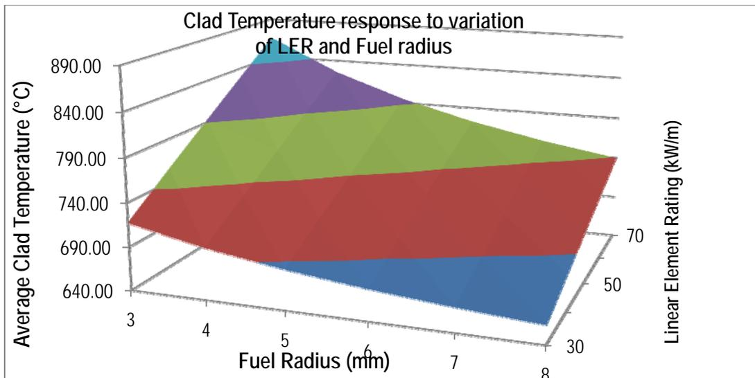
Figure 2 Clad Temperature with variation in LER and Fuel pellet radius
