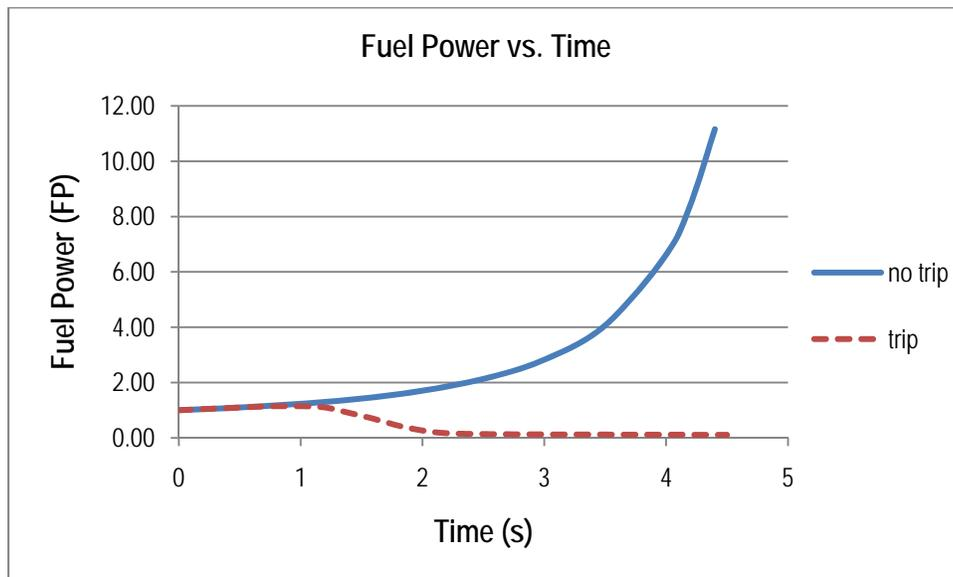
**Figure 10: Fuel Power vs. Time for 1 mk/s reactivity insertion rate**
