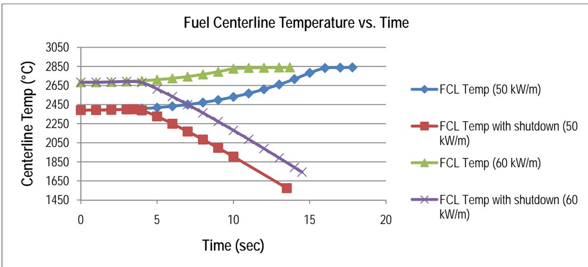
Figure 9: Fuel centerline temperature vs. time for 0.1 mk/s insertion rate
