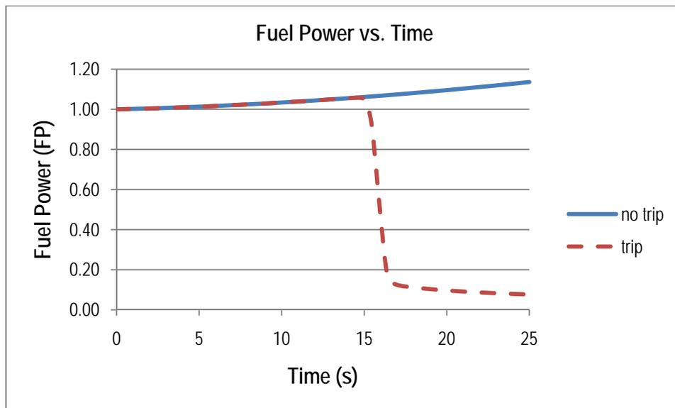
**Figure 4: Fuel Power vs. Time for 0.01 mk/s reactivity insertion rate**
