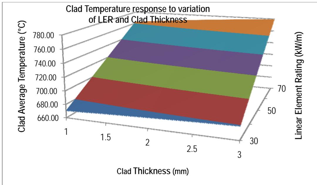
Figure 3: Clad Temperature with variation in LER and clad thickness
