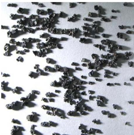
Fig. 4: HTF titanium filtration material
