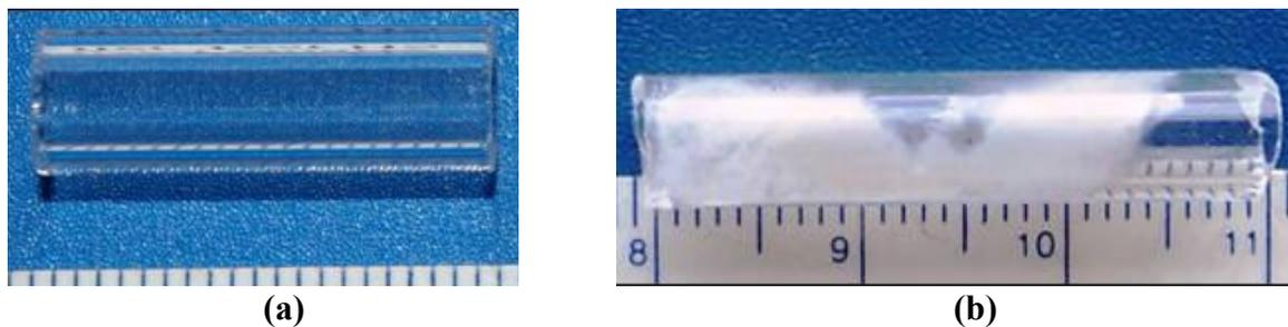
Figure 6 Silica glass samples after an exposure to (a) the Cu-Cl test environment and (b) the SI test environment (Items 9 and 11 in Table 4).
