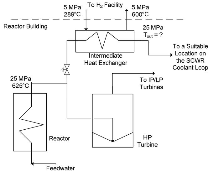
**Figure 1. Potential HX location for a no-reheat SCWR NPP layout.**
