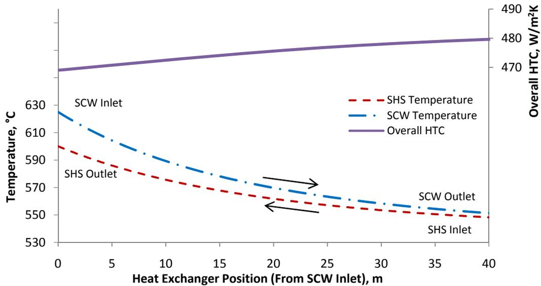
Figure 4. Temperature profiles obtained for excessive SHS flow.
