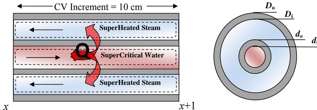
**Figure 2. Inner and outer pipes arrangement for a double-pipe HX (not to scale).**
