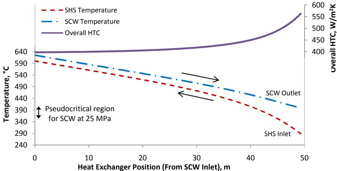
**Figure 3. Temperature profiles obtained using the heat balance method.**
