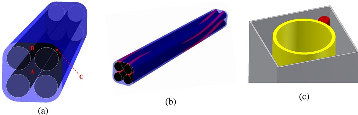
Figure 2 Three examples of geometries employed for the CFD analyses on heat transfer to super-critical water: (a) a four rod-bundle without wire-wrap, (b) a four rod-bundle with wire-wrap and (c) a square annulus with wire-wrap and cladding (c).
