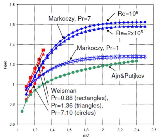
Figure 1 Rod bundle geometry factor  $F_{geo}$  as a function of pitch-to-diameter ratio  $p/d$  deduced from three common heat transfer correlations for rod-bundles in a square lattice arrangement.
