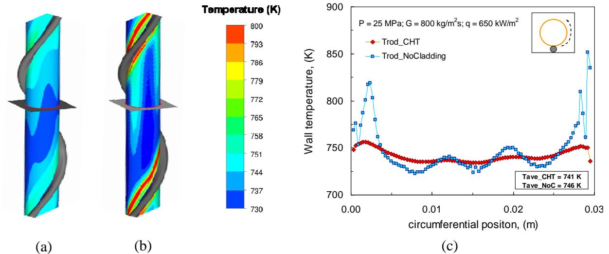
Figure 3 The effect of cladding for the wired square annulus. The calculated temperature contours over the fuel rod surface with and without cladding is shown in (a) and (b), respectively. The calculated temperature profiles over the fuel rod surface at a certain axial position are compared in (c).
