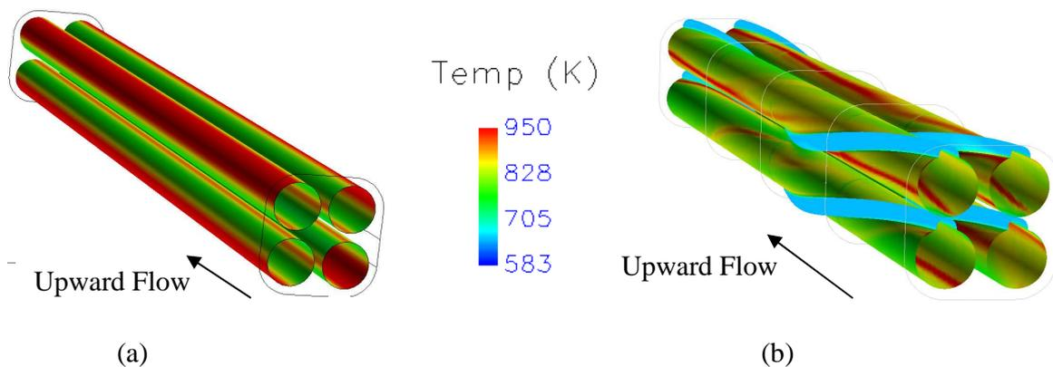
Figure 4 Calculated surface temperature contours on the fuel rods for an unwired (a) and wired (b) four rod-bundle assembly. Shown are the sections with an axial position between 1.6 and 1.8 m.
