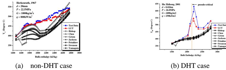
Figure 6. Comparison of test data with values predicted by the LUT and other for typical heat transfer cases
