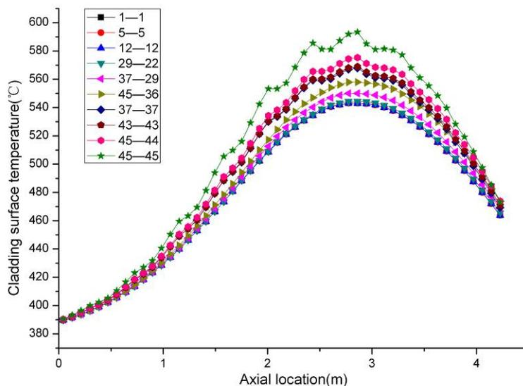
Figure 13 Axial cladding surface temperature of outer subchannel
