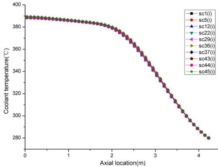
Figure 11 Axial coolant temperature distribution of inner subchannel
