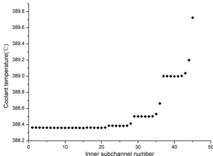
Figure 9 The outlet coolant temperature of inner subchannels
