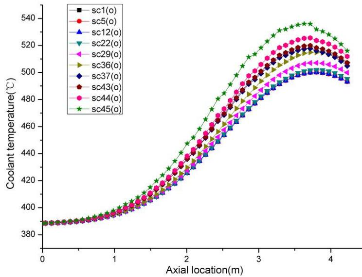
Figure 12 Axial coolant temperature distribution of outer subchannel
