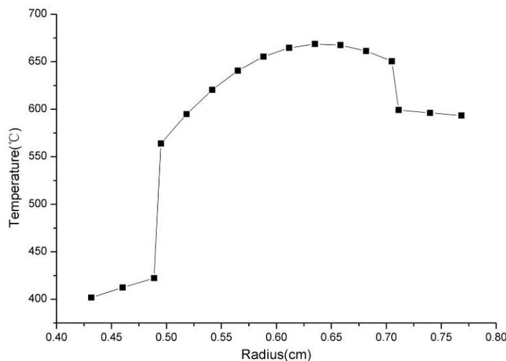
Figure 14 Radial fuel temperature distribution of the hotspot
