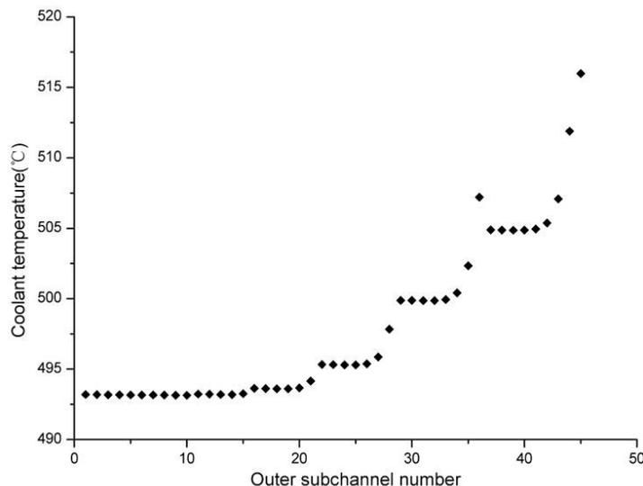
Figure 10 The outlet coolant temperature of outer subchannels
