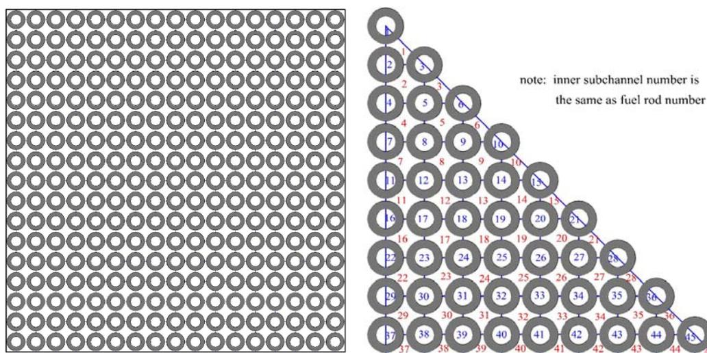
Figure 8 17×17 fuel assembly and subchannel identification in a 1/8 assembly
