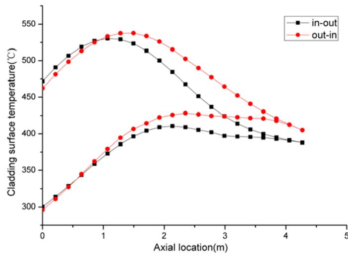
Figure 6 Axial distribution of cladding surface temperature
