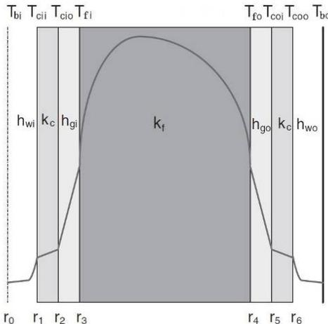
Figure 3 Radial temperature profile and node location
