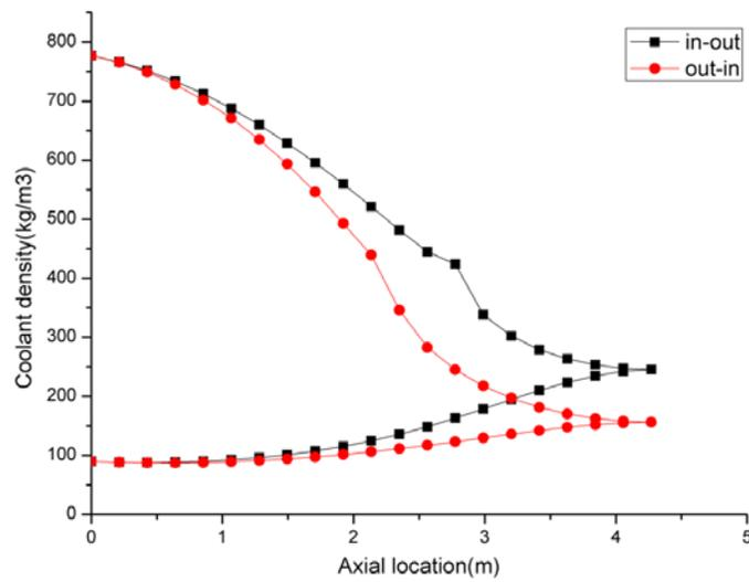
Figure 5 Axial distribution of coolant density
