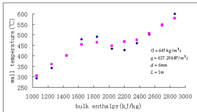
Fig.3 the comparison between the experiment data(red) and the value(black) calculated by the new correlation when heat transfer deterioration occurs.
