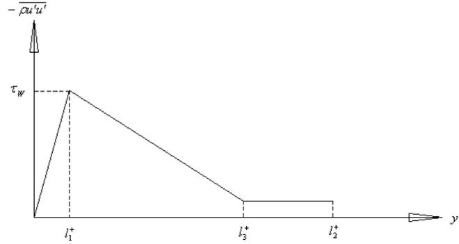
Fig.1 The distribution of Reynolds stress  $-\overline{\rho u' u'}$  along the normal position of wall
