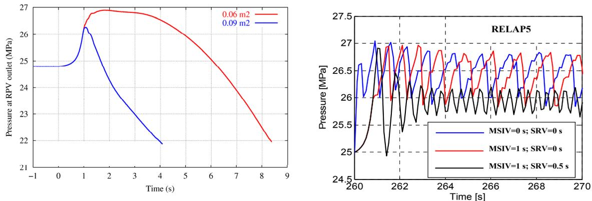
Figure 3 Pressure transient following a turbine trip calculated with the SMABRE/TRAB-3D (left) and RELAP5 (right) codes.
