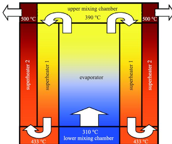
Figure 1 Three pass design concept of HPLWR core [3].
