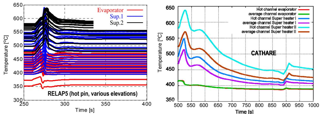
Figure 4 Peak cladding temperature calculated with the RELAP5 and CATHARE codes for a LOFW event, with failure of two pumps and delayed start-up of one stand-by pump.
