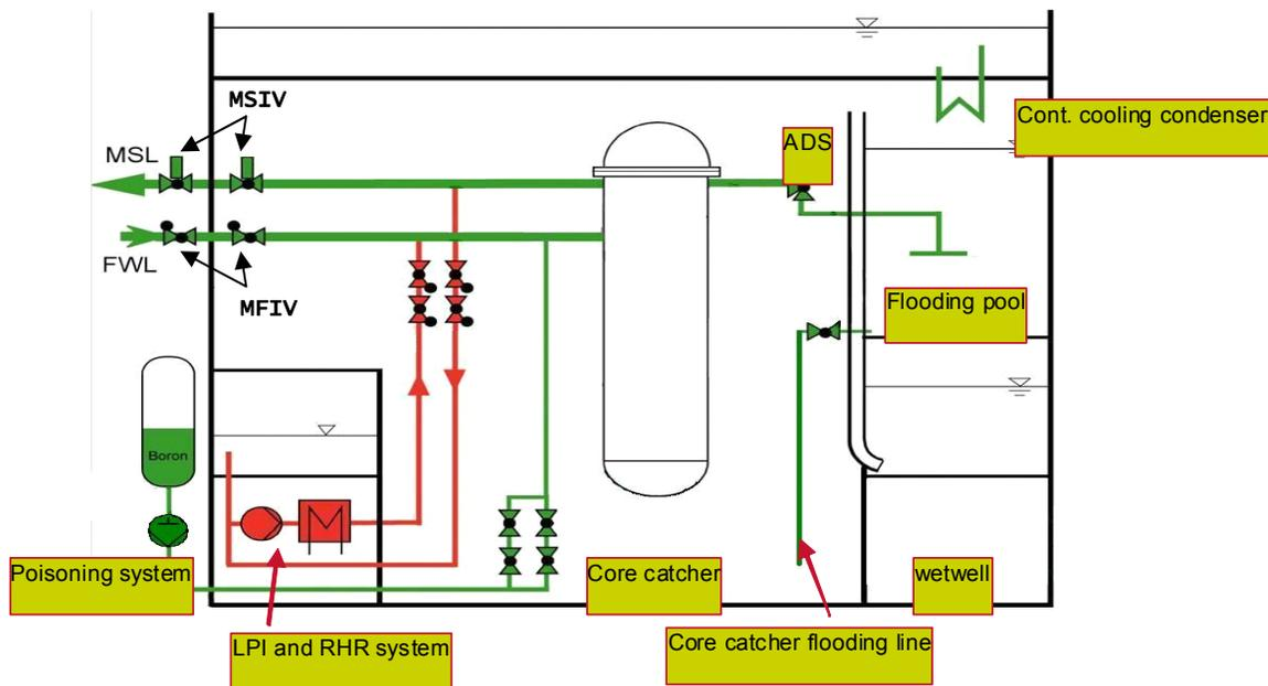
Figure 2 General configuration of the safety systems.
