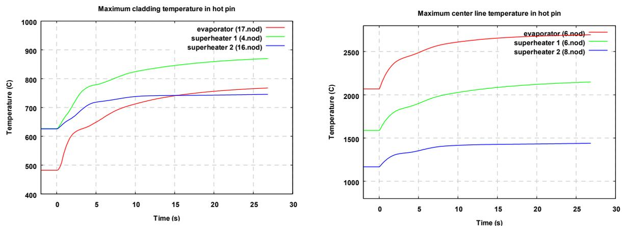
Figure 10 Peak cladding (left) and fuel (right) temperatures in the three regions of the core calculated by ATHLET-KIKO3D for a CRE with 0.1 s ejection time.
