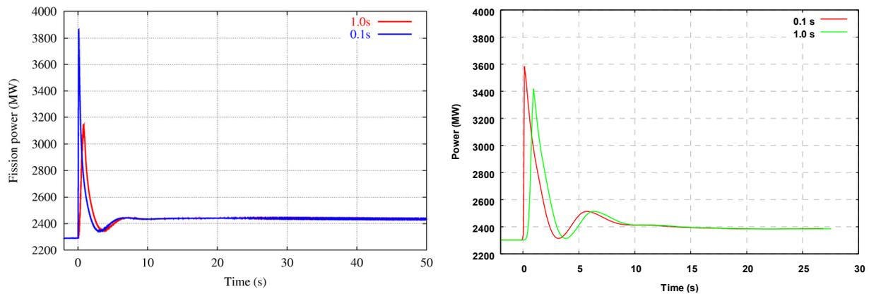
Figure 9 Comparison of the power calculated for a CRE event with SMABRE/TRAB-3D (left) and ATHLET-KIKO3D (right) for the two cases with 0.1 s and 1 s ejection time, respectively.
