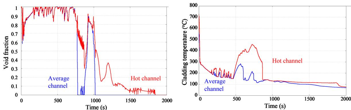
Figure 7 Average void fraction (right) and peak cladding temperature (right) in superheater 1 calculated by CATHARE for a large break in the feedwater line.
