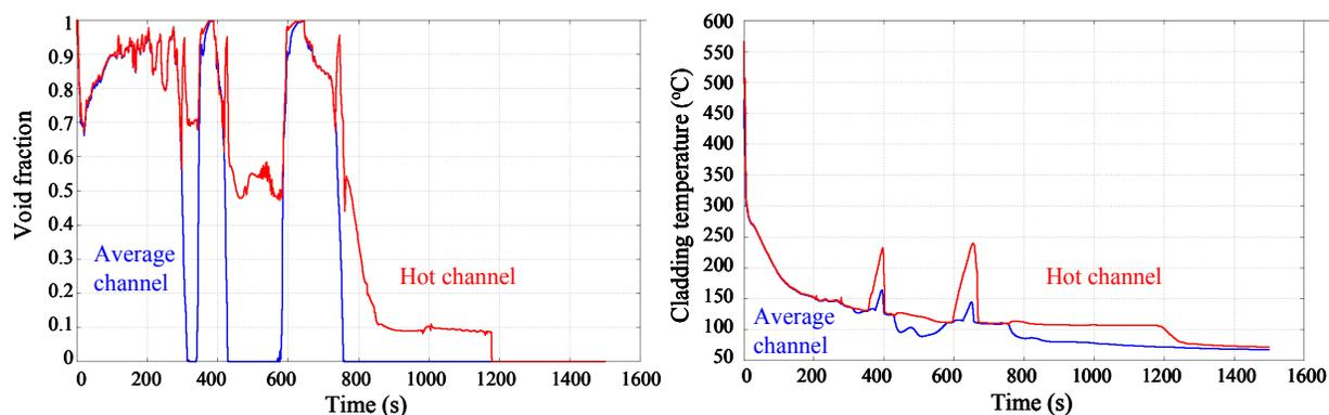
Figure 5 Average void fraction (left) and maximum cladding temperature (right) in superheater 1 calculated by CATHARE for a MSLB.
