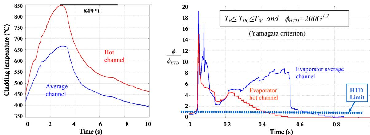
Figure 8 Peak cladding temperature in the evaporator calculated by CATHARE for a large LOCA in the feedwater line during the first seconds (left) and occurrence of heat transfer deterioration (right).
