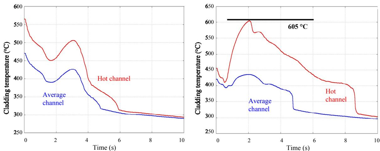
Figure 6 Peak cladding temperature in superheater 1 (left) and in the evaporator (right) during the first seconds of a MSLB calculated by CATHARE.
