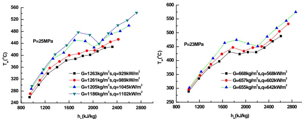
Fig.5 Heat transfer deterioration phenomenon in 25 and 23MPa
