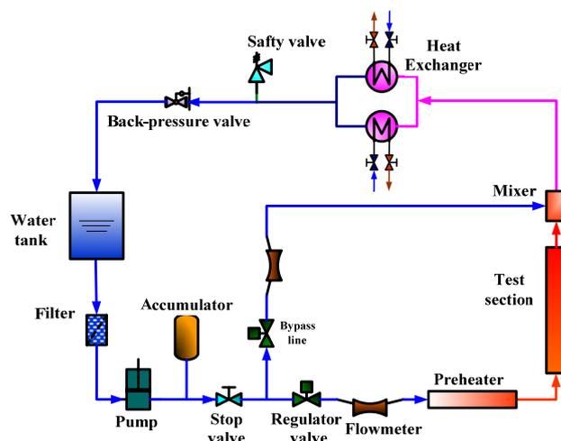
Fig.1 Schematic diagram of SCTM loop
