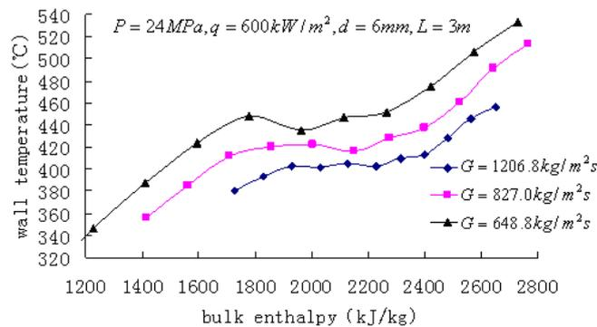
(b) Wall temperature at 24MPa, 600 kg/m<sup>2</sup>•s with different mass flux
