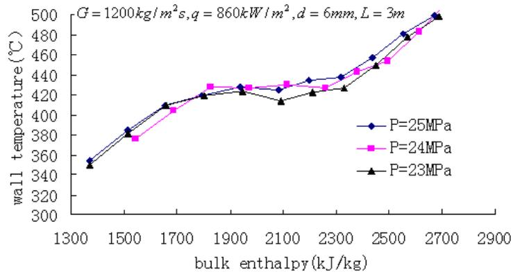
(c) Wall temperature at 860 kW/m<sup>2</sup>, 1200 kg/m<sup>2</sup>•s with different pressure
