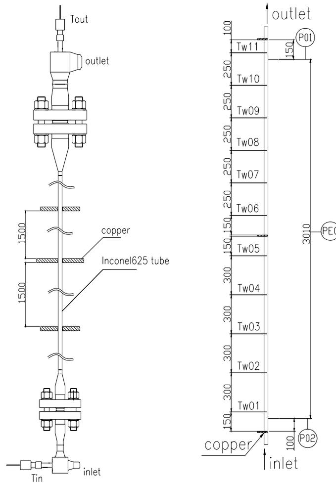
(a) detailed drawing of test section (b) measuring points distributing of test section
