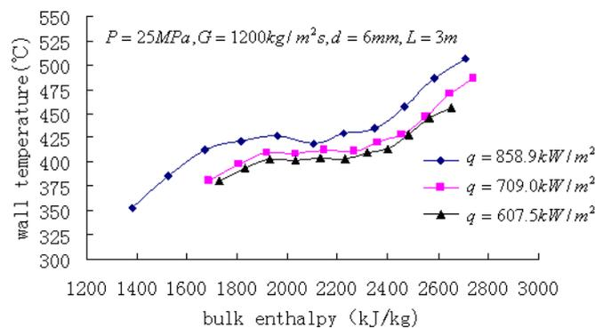
(a) Wall temperature at 25MPa, 1200 kg/m<sup>2</sup>•s with different heat flux
