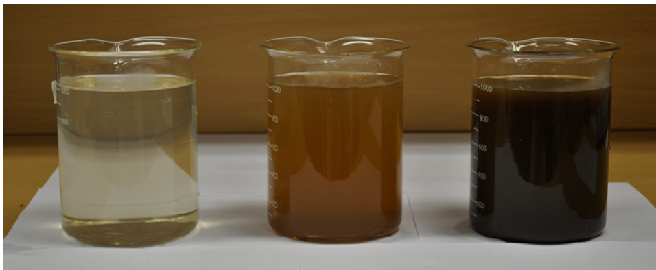
Figure 2 Well-dispersed magnetic nanofluids with concentrations of 1, 10 and 100 ppmv (from left to right)
