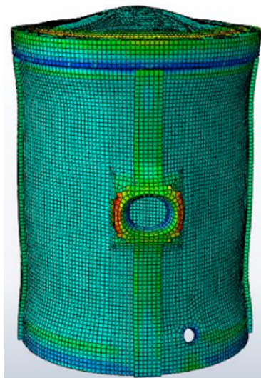
Figure 3 Stress distribution( 0P_{\text{design}} )
