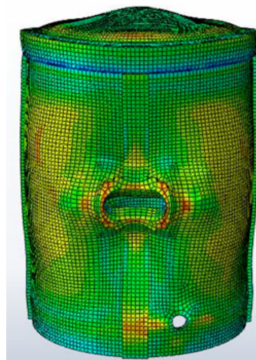
Figure 4 Stress distribution( 1.7P_{\text{design}} )
