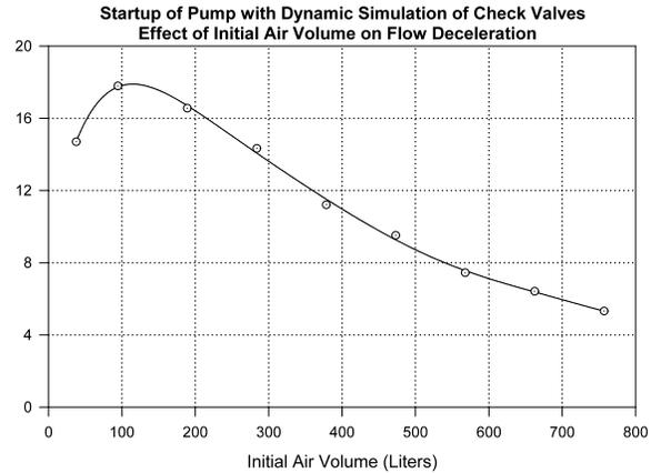
Figure 11 Effect of air on deceleration
