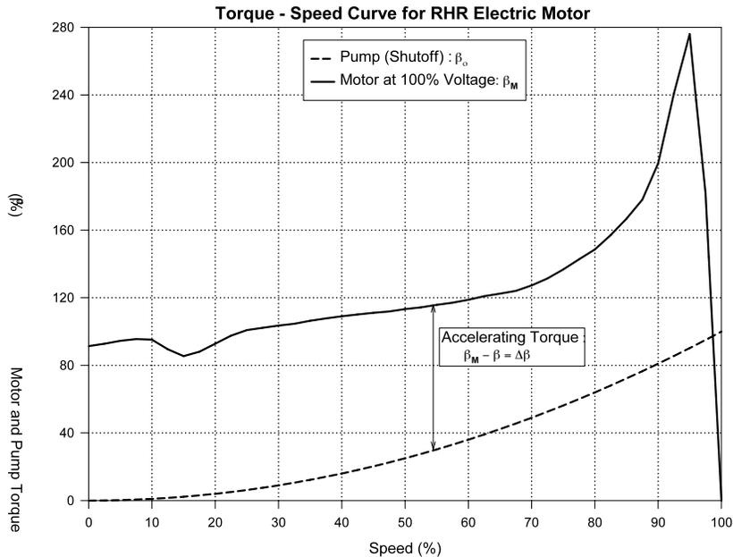
Figure 4 Torque-speed curve for motor
