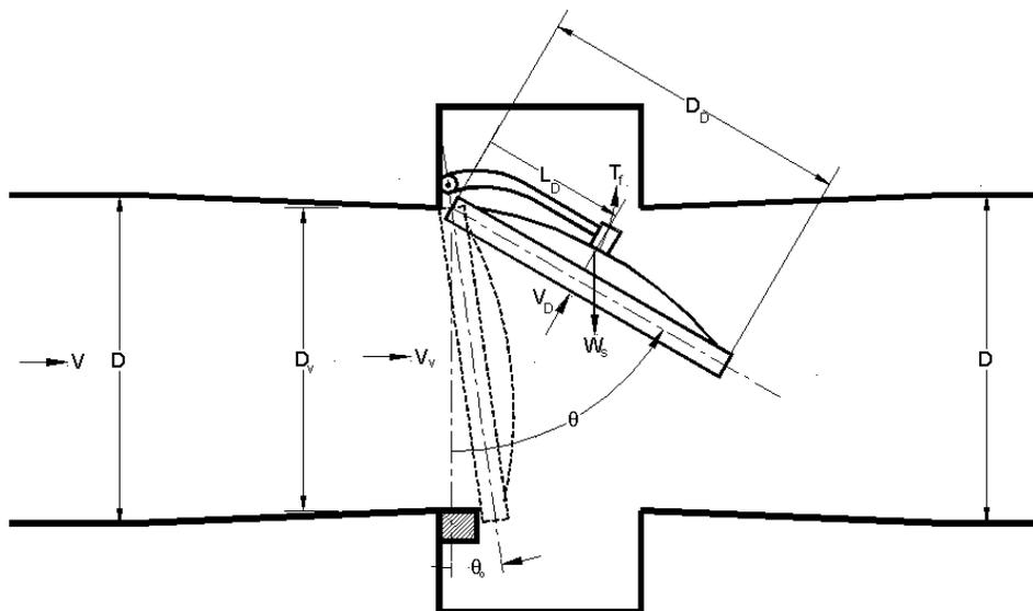
Figure 2 Diagram of check valve and definition of physical quantities
