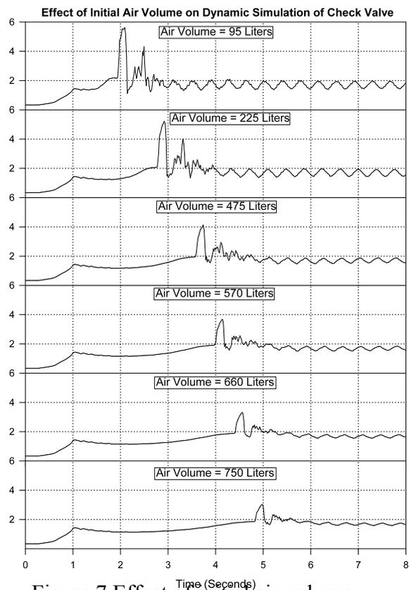
Figure 7 Effect of initial air volume
