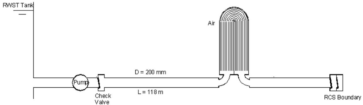
Figure 1 Schematic illustrating tank, piping, pump, check valve, and heat exchanger
