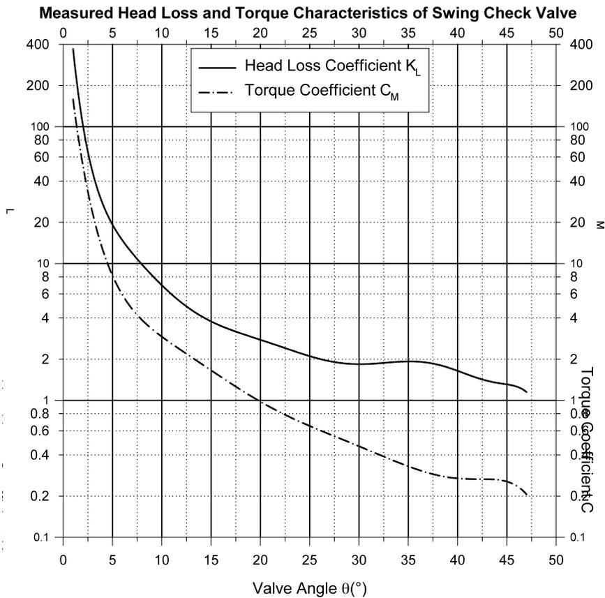
Figure 3 Coefficients of head loss  $K_L$  and torque  $C_M$  for swing check valve
