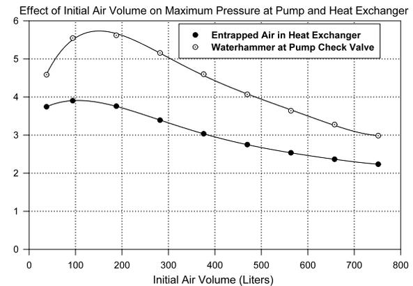
Figure 9 Effect of air volume on pressure
