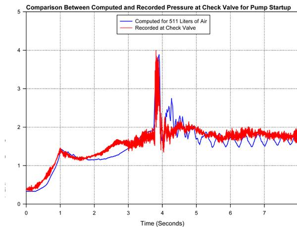
Figure 8 Pressure recording versus analysis
