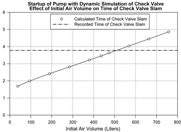
Figure 10 Effect of air on deceleration time
