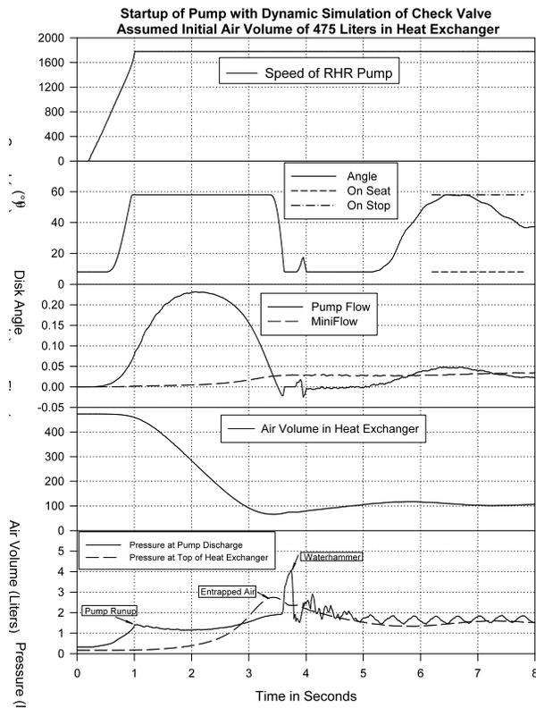
Figure 6 Simulation of check-valve slam with air
