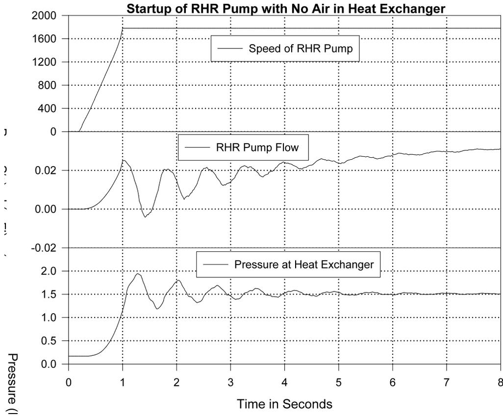
Figure 5 Simulation of pump startup with no air in heat exchanger
